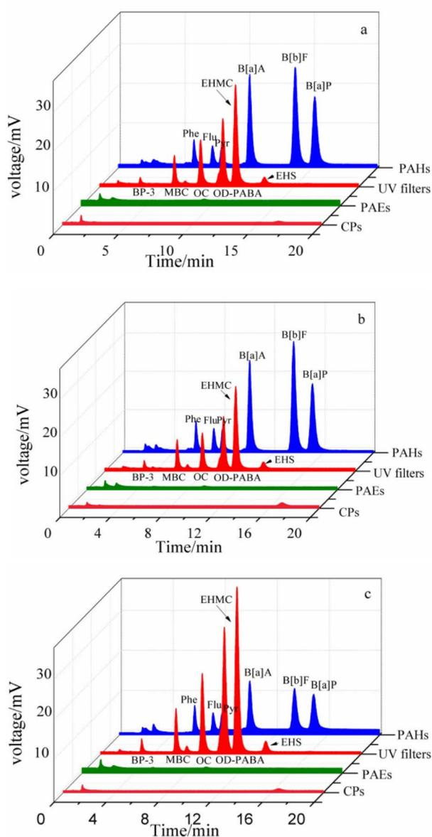
Fig. 6 SPME-HPLC chromatograms of (a) NiTi@NiTiONFs@ZIF-67-Co<sub>3</sub>O<sub>4</sub>, (b) NiTi@NiTiONFs@ZIF-67-C, and (c) NiTi@NiTiONFs@ZIF-67-NC.
