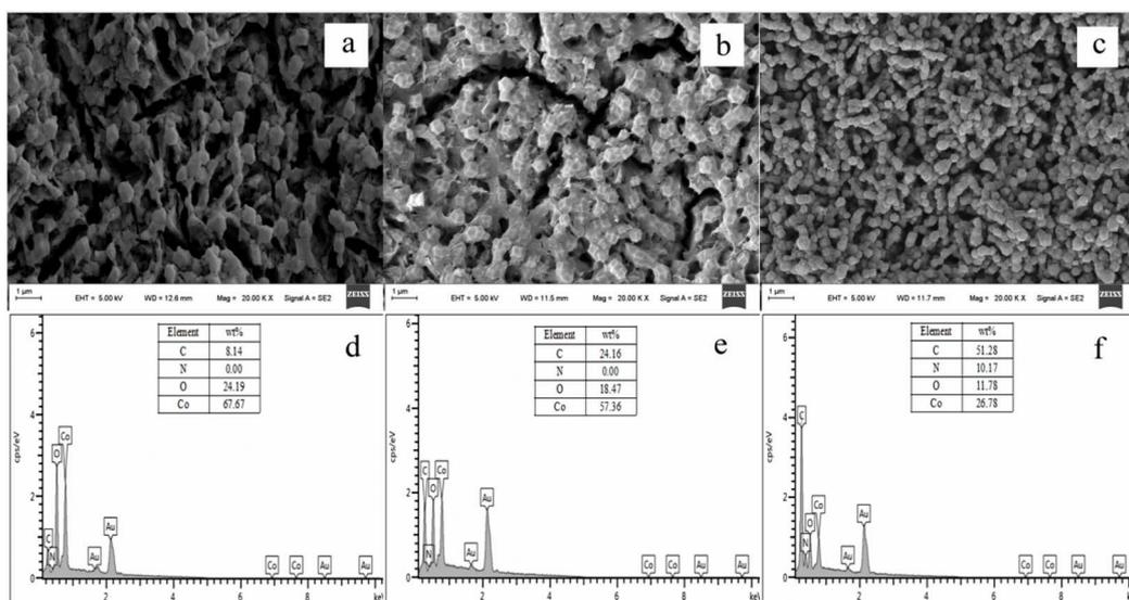
Fig. 5 SEM images (a–c) and EDS spectra with corresponding elemental compositions (d–f) of the ZIF-X (X = Co<sub>3</sub>O<sub>4</sub> (a and d), C (b and e), and NC (c and f)) coatings.
