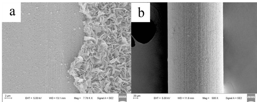
Fig. 2 SEM images of  $\text{Co(OH)}_2$  electrodeposited on different substrates (a) direct electrodeposition of  $\text{Co(OH)}_2$  coating on the bare NiTi wire; (b) electrodeposition of  $\text{Co(OH)}_2$  coating on the fiber after hydrothermal treatment with NaOH.
