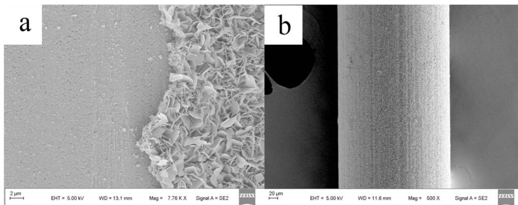
Fig. 2 SEM images of  $\text{Co(OH)}_2$  electrodeposited on different substrates (a) direct electrodeposition of  $\text{Co(OH)}_2$  coating on the bare NiTi wire; (b) electrodeposition of  $\text{Co(OH)}_2$  coating on the fiber after hydrothermal treatment with NaOH.
