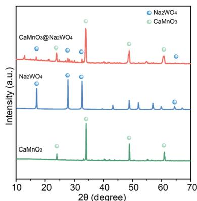
Fig. 1 XRD patterns of perovskite metal oxides  $\text{CaMnO}_3$  and  $\text{CaMnO}_3@Na_2WO_4$ .
