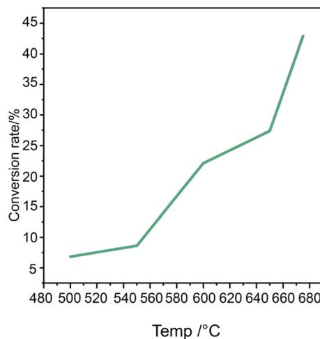
Fig. 4 Effect of reaction temperature on the conversion of the *n*-octane dehydrogenation reaction with CaMnO<sub>3</sub>@Na<sub>2</sub>WO<sub>4</sub> perovskite.
