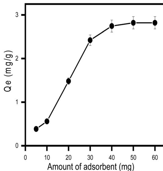
Fig. 6 Adsorption of 2,4,6-TCP on the AAES/GO composite as a function of amount [experimental conditions: the concentration of 2,4,6-TCP =  $10 \mu\text{g ml}^{-1}$ , contact time = 10 min, volume of test solution = 25 ml at pH = 6.5] Effect of initial concentration of 2,4,6-TCP.
