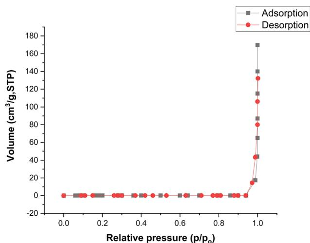
Fig. 5 Nitrogen adsorption–desorption isotherm of AAE/GO composite.
