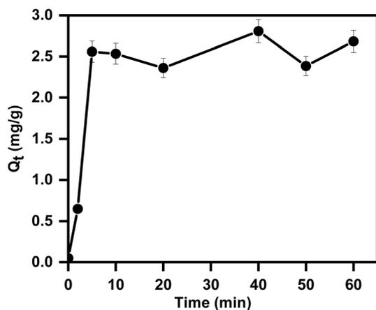
Fig. 9 Adsorption of 2,4,6-TCP on the AAES/GO composite as a function of time [experimental conditions: adsorbent dose = 40 mg, initial concentration =  $10 \mu\text{g ml}^{-1}$ , volume of test solution = 25 ml at pH = 6.5].
