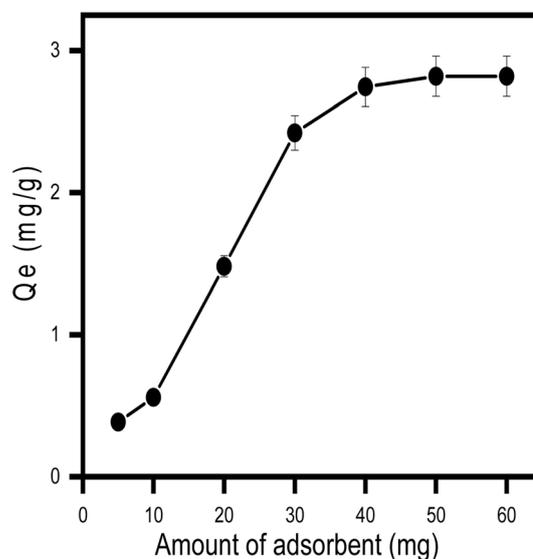
Fig. 6 Adsorption of 2,4,6-TCP on the AAES/GO composite as a function of amount [experimental conditions: the concentration of 2,4,6-TCP =  $10 \mu\text{g ml}^{-1}$ , contact time = 10 min, volume of test solution = 25 ml at pH = 6.5] Effect of initial concentration of 2,4,6-TCP.
