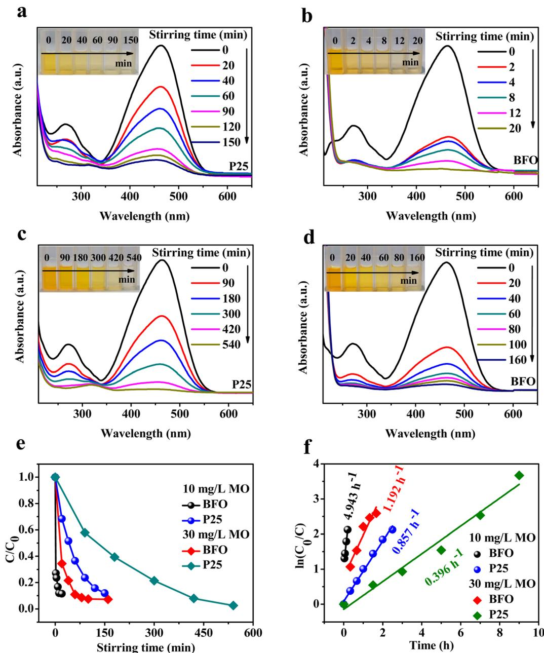
Fig. 2 Ultraviolet-visible absorption spectra of MO at different concentrations (inset: color contrast): (a) P25 10 mg L<sup>-1</sup>, (b) BFO 10 mg L<sup>-1</sup>, (c) P25 30 mg L<sup>-1</sup>, and (d) BFO 30 mg L<sup>-1</sup>. (e) Degradation rates and (f) kinetics curves of BFO and P25 powders at 10 mg L<sup>-1</sup> and 30 mg L<sup>-1</sup> concentrations.
