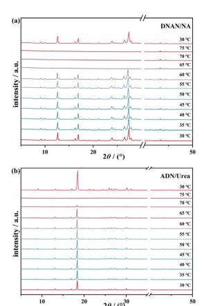
Fig. 3 (a) In situ XRD patterns of DNAN/NA cocrystal, (b) in situ XRD patterns of ADN/urea cocrystal.
