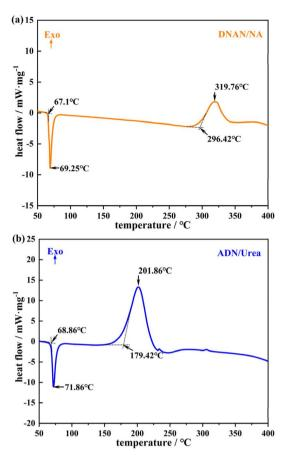
Fig. 2 (a) DSC curves of the DNAN/NA cocrystal, (b) DSC curves of the ADN/urea cocrystal
