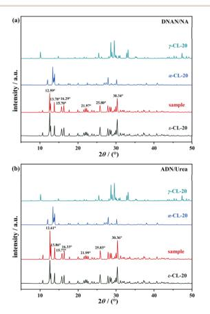
Fig. 5 (a) XRD patterns of  $\epsilon$ -CL-20 in DNAN/NA carrier, (b) XRD patterns of  $\epsilon$ -CL-20 in ADN/urea carrier.
