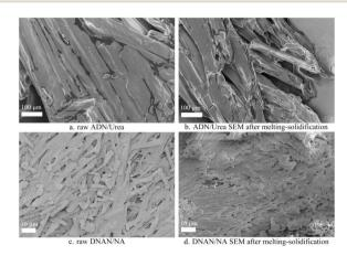
Fig. 4 SEM of ADN/urea and DNAN/NA cocrystals.
