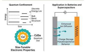
Fig. 1 Schematic of quantum confinement and size-dependent electrochemical properties in CdSe QDs for energy storage applications.
