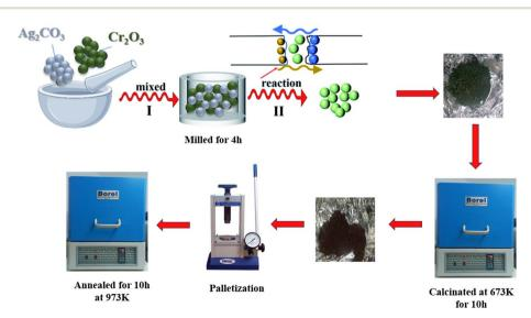
Fig. 1 Schematic diagram showing the different steps of the solid-state reaction method followed for the synthesis of AqCrO<sub>2</sub> compound.
