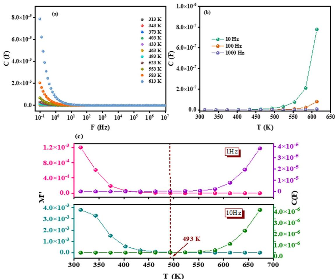
Fig. 16 Variation capacitance with frequencies (a), evolution of capacitance versus temperature for selective frequencies (b). Variation both of imaginary part of the electrical modulus  $M''$  and capacitance versus temperature for selective frequencies (c).
