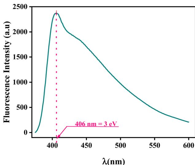
Fig. 6 Fluorescence emission spectrum of the  $\text{AgCrO}_2$  compound.
