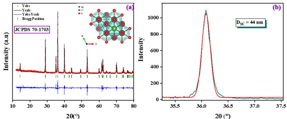
Fig. 2 (a) Observed, and calculated X-ray powder diffraction patterns and reflection positions are marked for the phase. Inset projection crystal structure *c*-axis. (b) Selection of the highest peak in the X-ray diffraction pattern for the determination of crystallite size using the Scherrer equation.
