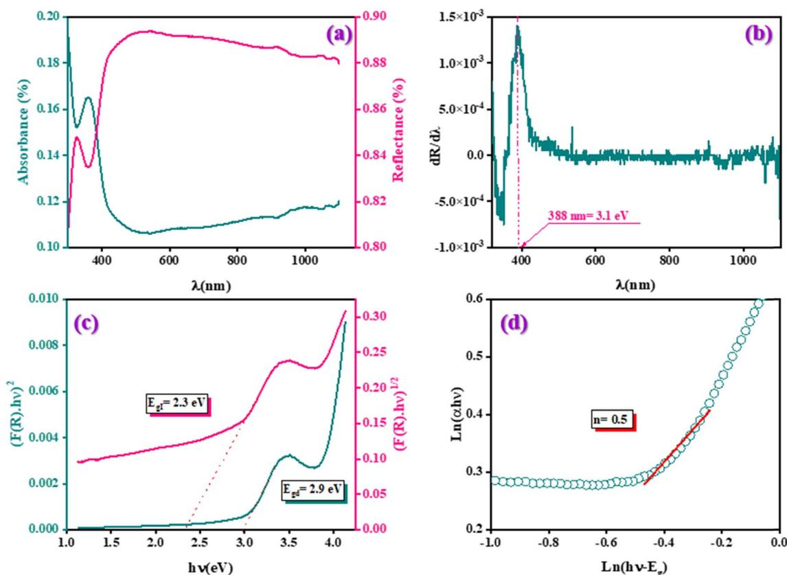
Fig. 4 (a) UV-Vis absorbance and reflectance spectrum at room temperature, (b) evolution of  $dR/d\lambda$  as a function of  $\lambda$ , (c) the evolution of  $\ln(\alpha hv)$  against  $\ln(hv - E_g)$ , (d) plot of  $n(F(R) \times hv)^2$  and  $(F(R) \times hv)^{1/2}$  versus  $hv$ .
