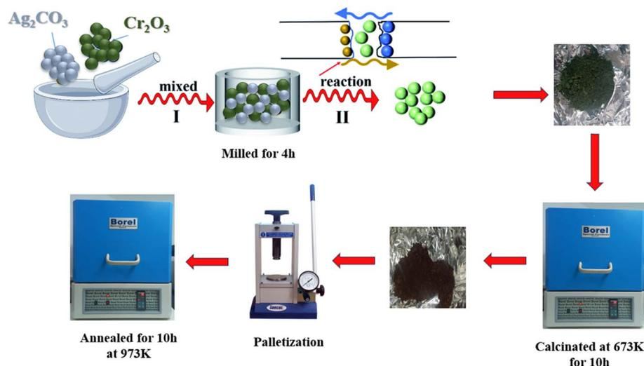
Fig. 1 Schematic diagram showing the different steps of the solid-state reaction method followed for the synthesis of AgCrO<sub>2</sub> compound.
