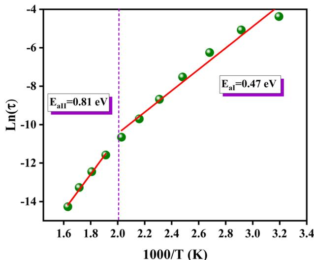
Fig. 14 Variation of  $\ln(\tau)$  as a function of  $1000/T$  for the compound  $\text{AgCrO}_2$ .
