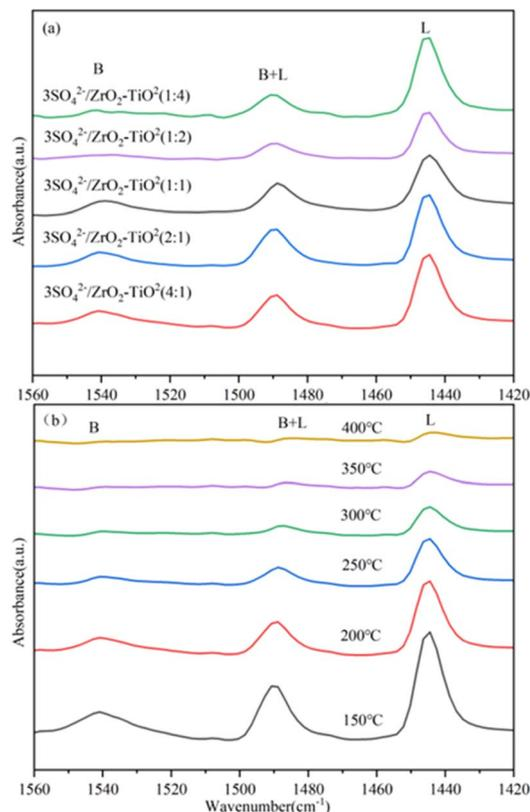
Fig. 6 Py-FTIR spectra of  $\text{SO}_4^{2-}/\text{ZrO}_2\text{-TiO}_2$  catalyst, (a) desorption spectra of different catalysts at 200 °C, (b) desorption spectra of  $\text{SO}_4^{2-}/\text{ZrO}_2\text{-TiO}_2$  (4 : 1) catalyst at different temperatures.
