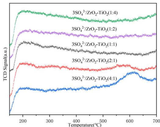
Fig. 5  $\text{NH}_3$ -TPD profiles of prepared catalysts.
