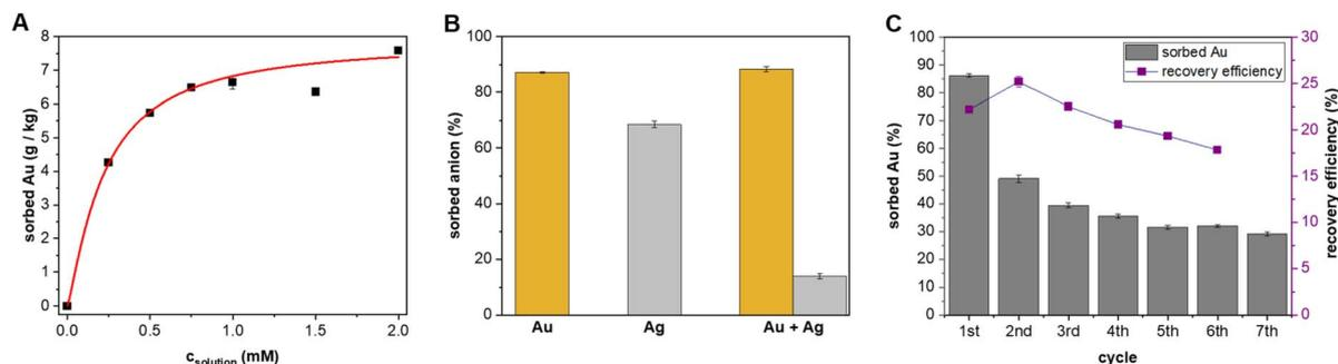
Fig. 2 (A) Langmuir-type isotherm of sorption. (B) Weight fraction of gold/silver removed from 1 mM water solution of K[Au(CN)<sub>2</sub>], K[Ag(CN)<sub>2</sub>], and the mixture of both anions by the SG-BU (9 : 1) material (100 mg). (C) Sorption efficiency (weight fraction of gold removed from 1 mM water solution of K[Au(CN)<sub>2</sub>]) and recovery efficiency (weight fraction of gold removed from the SG-BU (9 : 1) material after treatment with NaCl solution) during several recycling steps.
