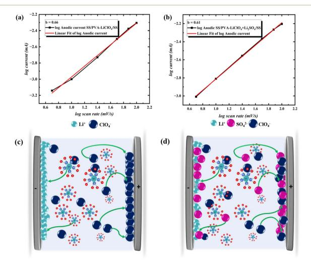
Fig. 6 (a) Dual logarithm plot of current *versus* scan rate of CV in SS $\parallel$ PVA-LiClO<sub>4</sub> $\parallel$ SS, (b) dual logarithm plot of current *versus* scan rate of CV in SS $\parallel$ PVA-LiClO<sub>4</sub> + Li<sub>2</sub>SO<sub>4</sub> $\parallel$ SS, (c) deposition of Li<sup>+</sup> in the electrode surface, (d) inhibition of further Li<sup>+</sup> deposition by SO<sub>4</sub><sup>2-</sup>.
