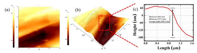
Fig. 4 (a) 2D AFM image of the thin film (b), 3D image (c) height profile (thickness) of the film.
