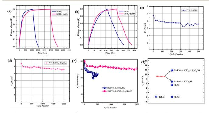
Fig. 3 (a) GCD 1st cycle at 0.5 microampere (b)  $1^{st}$  cycle at 1 microampere, (c) cyclic stability of SS||PVA-LiClO<sub>4</sub>||SS (d) cyclic stability SS||PVA-LiClO<sub>4</sub> + Li<sub>2</sub>SO<sub>4</sub>||SS (e) comparison of  $C_V$  retention of both devices (f) comparison with previous literature.
