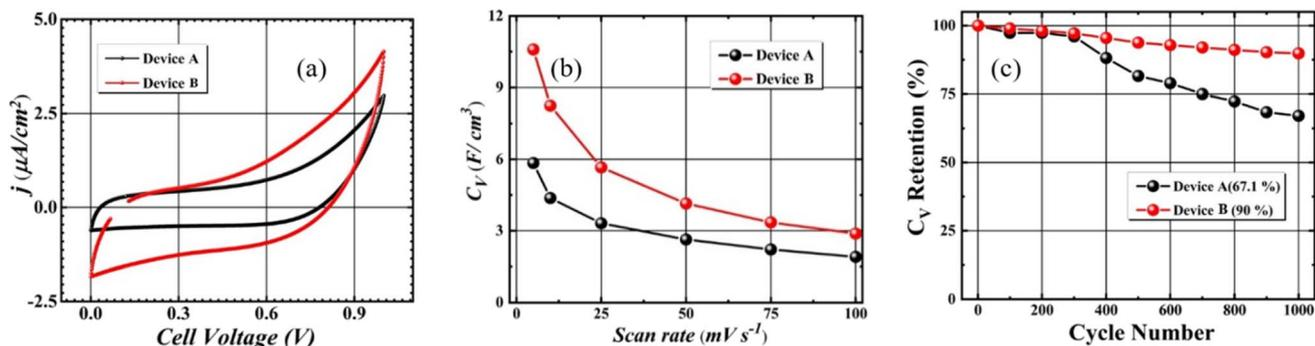
Fig. 2 (a) Stability performance of device A (SS||PVA-LiClO<sub>4</sub>||SS) and B (SS||PVA-LiClO<sub>4</sub> + Li<sub>2</sub>SO<sub>4</sub>||SS), (b) C<sub>V</sub> comparison of device A and B, (c) C<sub>V</sub> comparison at 10 mV s<sup>-1</sup> scan rate of device SS||PVA-LiClO<sub>4</sub> + Li<sub>2</sub>SO<sub>4</sub>||SS (A) and SS||PVA-LiClO<sub>4</sub> + Li<sub>2</sub>SO<sub>4</sub>||SS (B).
