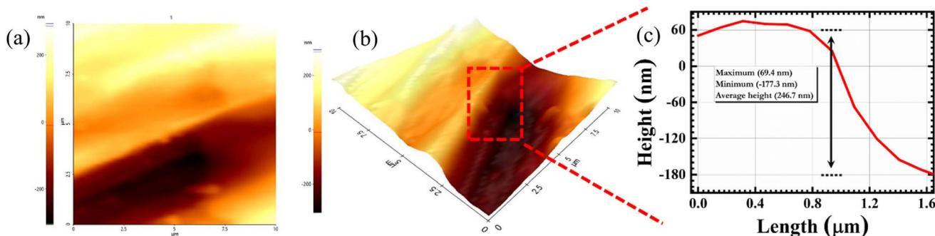
Fig. 4 (a) 2D AFM image of the thin film (b), 3D image (c) height profile (thickness) of the film.
