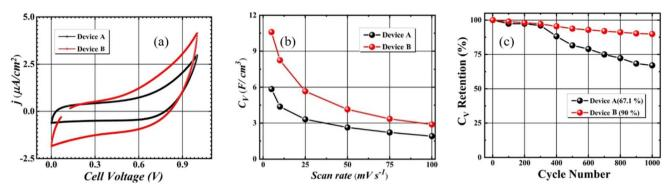
Fig. 2 (a) Stability performance of device A (SS||PVA-LiClO<sub>4</sub>||SS) and B (SS||PVA-LiClO<sub>4</sub> + Li<sub>2</sub>SO<sub>4</sub>||SS), (b)  $C_V$  comparison of device A and B, (c)  $C_V$  comparison at 10 mV s<sup>-1</sup> scan rate of device SS||PVA-LiClO<sub>4</sub> + Li<sub>2</sub>SO<sub>4</sub>||SS (A) and SS||PVA-LiClO<sub>4</sub> + Li<sub>2</sub>SO<sub>4</sub>||SS (B).
