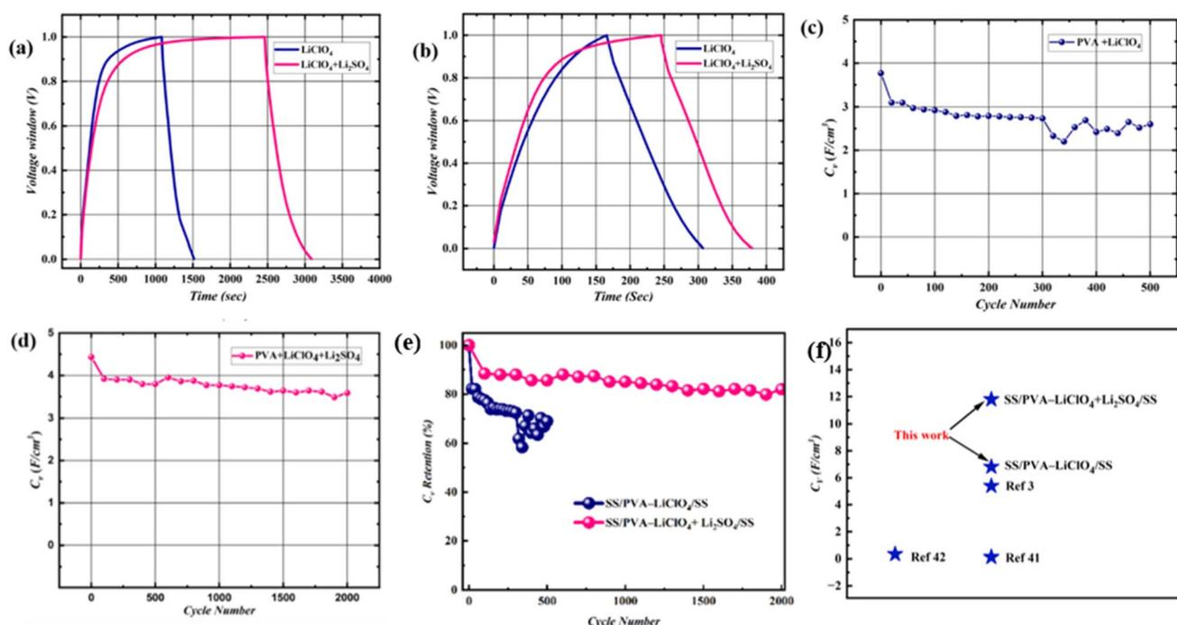
Fig. 3 (a) GCD 1st cycle at 0.5 microampere (b) 1<sup>st</sup> cycle at 1 microampere, (c) cyclic stability of SS||PVA-LiClO<sub>4</sub>||SS (d) cyclic stability SS||PVA-LiClO<sub>4</sub> + Li<sub>2</sub>SO<sub>4</sub>||SS (e) comparison of C<sub>V</sub> retention of both devices (f) comparison with previous literature.
