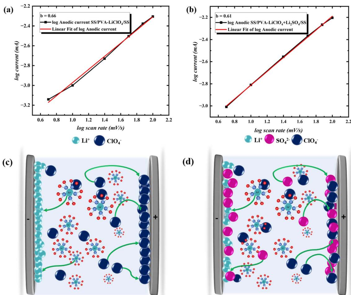
Fig. 6 (a) Dual logarithm plot of current versus scan rate of CV in SS||PVA-LiClO<sub>4</sub>||SS, (b) dual logarithm plot of current versus scan rate of CV in SS||PVA-LiClO<sub>4</sub> + Li<sub>2</sub>SO<sub>4</sub>||SS, (c) deposition of Li<sup>+</sup> in the electrode surface, (d) inhibition of further Li<sup>+</sup> deposition by SO<sub>4</sub><sup>2-</sup>.
