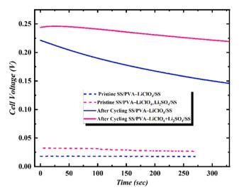
Fig. 5 Time-dependent  $V_{\rm cell}$  of SS||PVA-LiClO<sub>4</sub>||SS and SS||PVA-LiClO<sub>4</sub> + Li<sub>2</sub>SO<sub>4</sub>||SS measured as a function of time under pristine state v/s after cycling.
