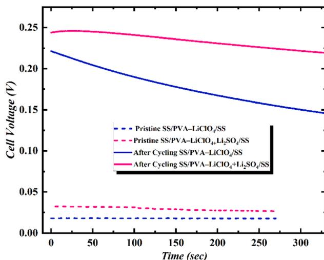
Fig. 5 Time-dependent  $V_{\text{cell}}$  of SS||PVA-LiClO<sub>4</sub>||SS and SS||PVA-LiClO<sub>4</sub> + Li<sub>2</sub>SO<sub>4</sub>||SS measured as a function of time under pristine state v/s after cycling.
