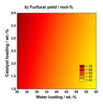
Fig. 1 DoE study for optimizing furfural yield depending on the relationship of reaction time vs. temperature (a) and catalyst loading vs. water loading (b). Reaction conditions: 0.25 g substrate, 5 g [DMBA] [HSO<sub>4</sub>] including deionized water, H<sub>4</sub>SiW<sub>12</sub>O<sub>40</sub> (HSiW).
