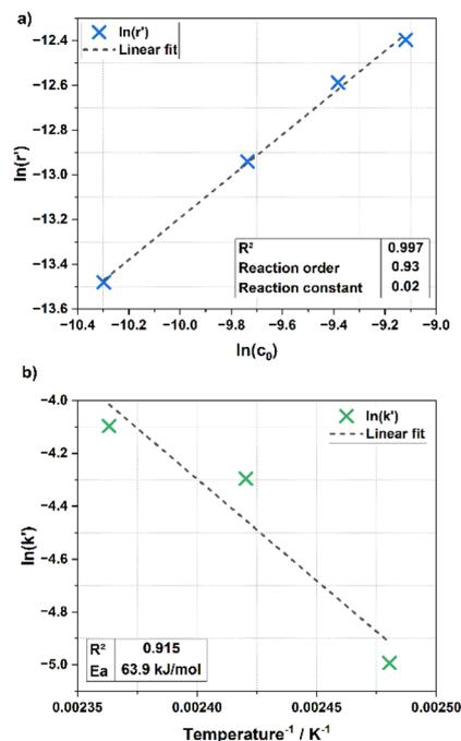
Fig. 2 Determination of reaction order (a) and activation energy (b). Reaction conditions (a): 0.1; 0.175; 0.25; 0.325 g (b) 0.25 g sugarcane bagasse, 5 g [DMBA][H<sub>2</sub>SO<sub>4</sub>] (including 20 wt% H<sub>2</sub>O), 0.20 g H<sub>4</sub>SiW<sub>12</sub>O<sub>40</sub> (HSiW),  $t = 90 \text{ min}$ ,  $T =$  (a) 150 °C (b) 130; 140; 150 °C.
