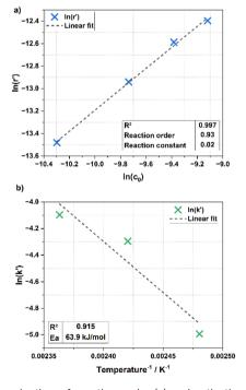
Fig. 2 Determination of reaction order (a) and activation energy (b). Reaction conditions (a): 0.1; 0.175; 0.25; 0.325 g (b) 0.25 g sugarcane bagasse, 5 g [DMBA][HSO<sub>4</sub>] (including 20 wt% H<sub>2</sub>O), 0.20 g H<sub>4</sub>SiW<sub>12</sub>O<sub>40</sub> (HSiW), t=90 min, T= (a) 150 °C (b) 130; 140; 150 °C.
