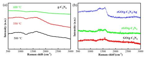
Fig. 8 Raman spectra of  $q-C_xN_4$  sheets prepared at different temperatures (a), and  $GO/q-C_xN_4$ ,  $rGO/q-C_xN_4$  and  $rGO/q-C_xN_4$ /Aq NPs (b).
