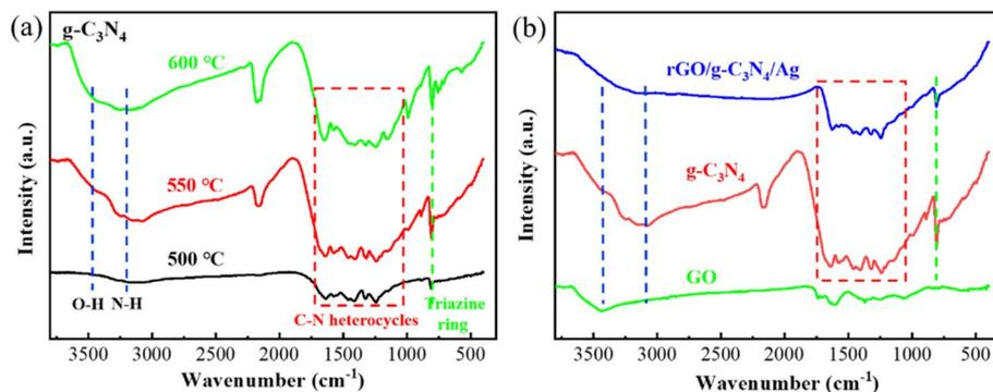
Fig. 7 FTIR spectra of  $g\text{-C}_3\text{N}_4$  sheets prepared at different temperatures (a), and FTIR spectra of GO,  $g\text{-C}_3\text{N}_4$  and  $r\text{GO}/g\text{-C}_3\text{N}_4/\text{Ag}$  NPs (b).
