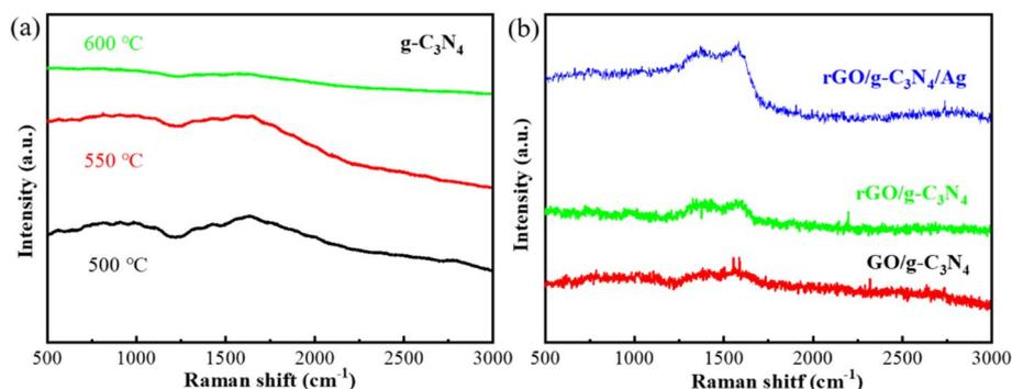
Fig. 8 Raman spectra of  $g\text{-C}_3\text{N}_4$  sheets prepared at different temperatures (a), and  $\text{GO}/g\text{-C}_3\text{N}_4$ ,  $r\text{GO}/g\text{-C}_3\text{N}_4$  and  $r\text{GO}/g\text{-C}_3\text{N}_4/\text{Ag}$  NPs (b).
