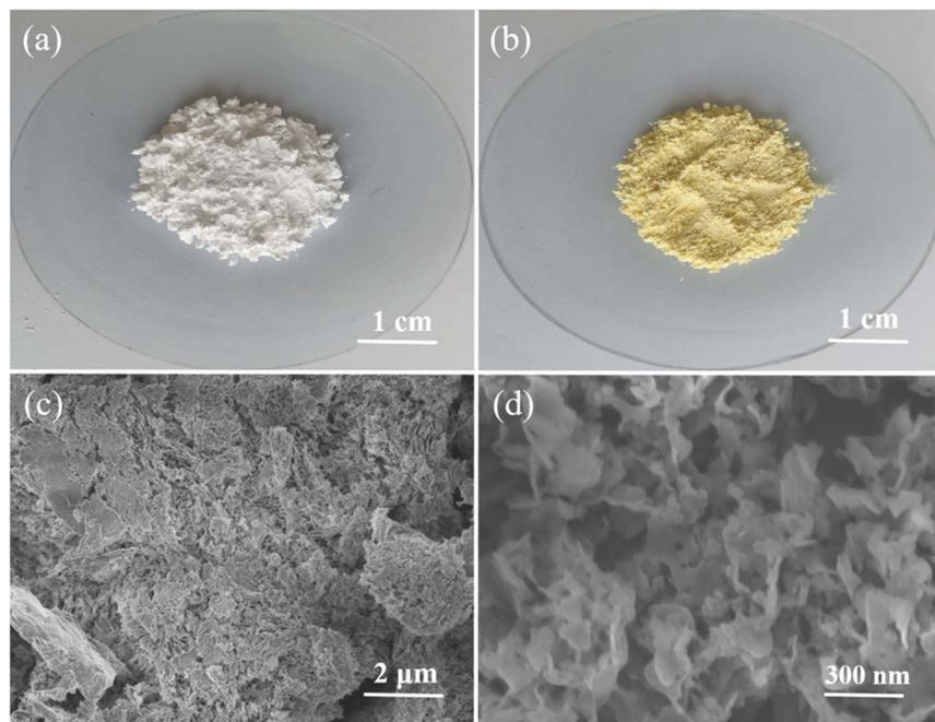
Fig. 3 Optical photos of melamine powders (a) and g-C<sub>3</sub>N<sub>4</sub> powders (b). SEM images of g-C<sub>3</sub>N<sub>4</sub> powders (c) and g-C<sub>3</sub>N<sub>4</sub> sheets (d).
