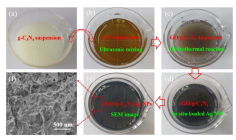
Fig. 1 A peparation schematic illustration of rGO/g- $C_3N_4$ /Ag NPs. Optical photos of aqueous suspensions of g- $C_3N_4$  (a), GO (b), GO/g- $C_3N_4$ /Ag NPs (c), rGO/g- $C_3N_4$ /Ag NPs (d), and rGO/g- $C_3N_4$ /Ag NPs (e). SEM image of rGO/g- $C_3N_4$ /Ag NPs (f).
