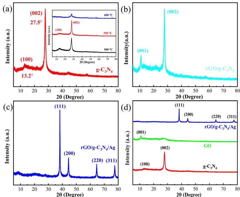
Fig. 9 XRD patterns of (a)  $g\text{-C}_3\text{N}_4$  sheets prepared at 550 °C, (b)  $r\text{GO}/g\text{-C}_3\text{N}_4$ , (c)  $r\text{GO}/g\text{-C}_3\text{N}_4/\text{Ag}$  NPs and (d)  $g\text{-C}_3\text{N}_4$ , GO and  $r\text{GO}/g\text{-C}_3\text{N}_4/\text{Ag}$  NPs. The inset of (a) is XRD patterns of  $g\text{-C}_3\text{N}_4$  sheets prepared at different temperatures.
