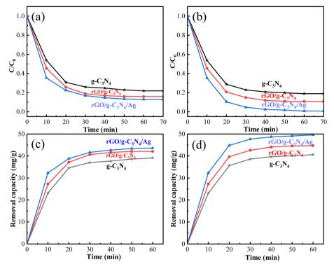
Fig. 10 The ratio of temporal concentration to initial concentration ( $C/C_0$ ) with the change of adsorption time (a) in the dark and (b) under visible light. MB removal capacity with the change of adsorption time (c) in the dark and (d) under visible light.
