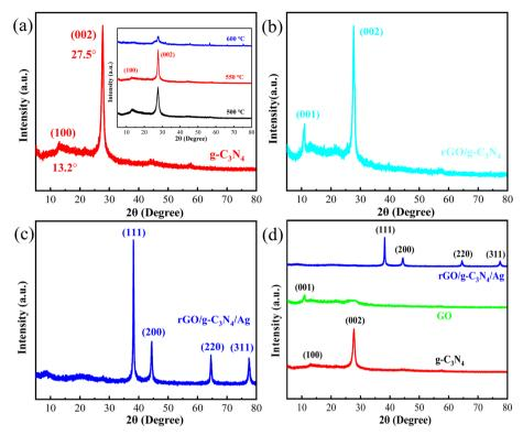
Fig. 9 XRD patterns of (a)  $g-C_3N_4$  sheets prepared at 550 °C, (b)  $rGO/g-C_3N_4$ , (c)  $rGO/g-C_3N_4/Ag$  NPs and (d)  $g-C_3N_4$ , GO and  $rGO/g-C_3N_4/Ag$  NPs. The inset of (a) is XRD patterns of  $g-C_3N_4$  sheets prepared at different temperatures.
