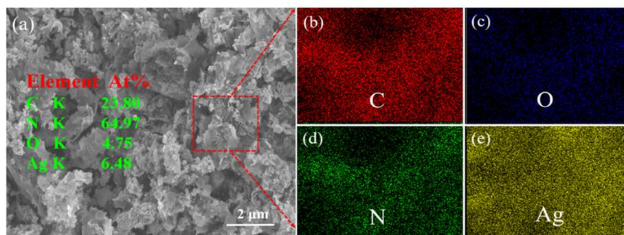
Fig. 6 (a) SEM image of rGO/g-C<sub>3</sub>N<sub>4</sub>/Ag NPs in a selected region, and (b–e) Elemental mappings of C, O, N and Ag.
