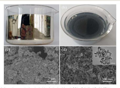
Fig. 4 Optical photos of silver mirror attached to the inside of a beaker (a) and rGO/g-C<sub>3</sub>N<sub>4</sub>/Ag NPs (b). SEM images of Ag NPs with different magnifications (c and d). The inset of (d) is TEM image of Ag NPs.
