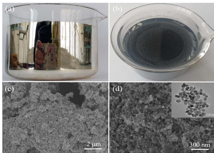
Fig. 4 Optical photos of silver mirror attached to the inside of a beaker (a) and rGO/g-C<sub>3</sub>N<sub>4</sub>/Ag NPs (b). SEM images of Ag NPs with different magnifications (c and d). The inset of (d) is TEM image of Ag NPs.
