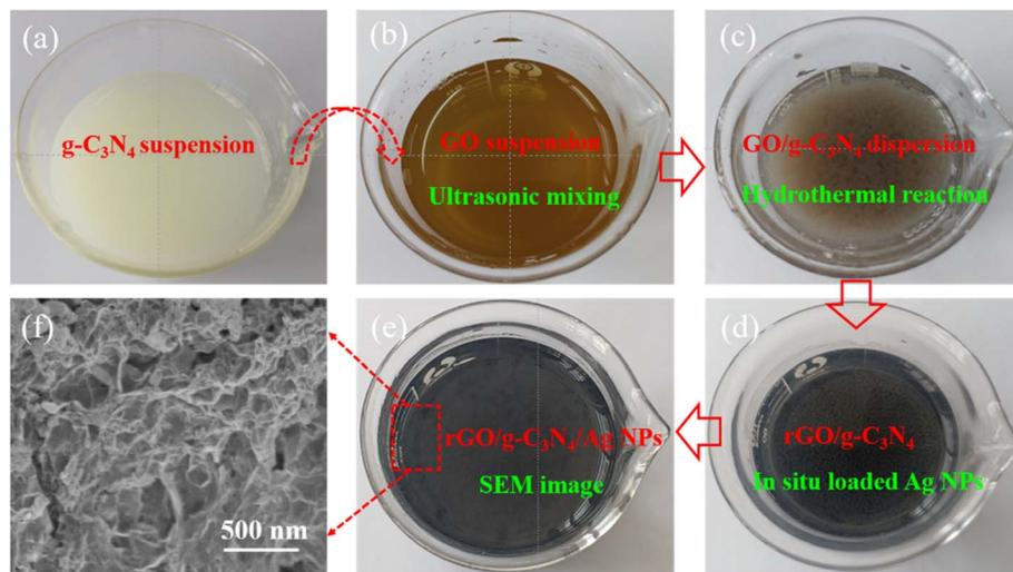
Fig. 1 A preparation schematic illustration of rGO/g-C<sub>3</sub>N<sub>4</sub>/Ag NPs. Optical photos of aqueous suspensions of g-C<sub>3</sub>N<sub>4</sub> (a), GO (b), GO/g-C<sub>3</sub>N<sub>4</sub> (c), rGO/g-C<sub>3</sub>N<sub>4</sub> (d), and rGO/g-C<sub>3</sub>N<sub>4</sub>/Ag NPs (e). SEM image of rGO/g-C<sub>3</sub>N<sub>4</sub>/Ag NPs (f).
