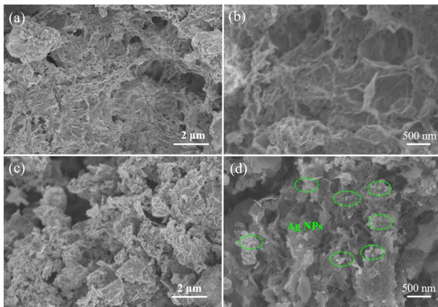
Fig. 5 SEM images of rGO/g-C<sub>3</sub>N<sub>4</sub> nanocomposite with different magnifications (a and b), and rGO/g-C<sub>3</sub>N<sub>4</sub>/Ag NPs with different magnifications (c and d).
