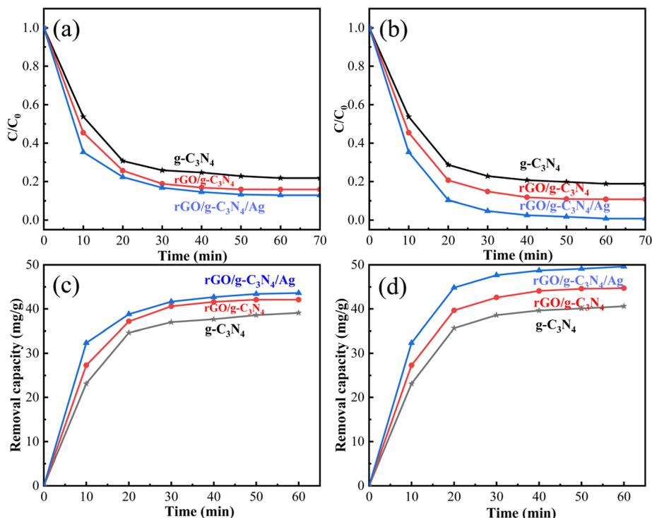
Fig. 10 The ratio of temporal concentration to initial concentration ( $C/C_0$ ) with the change of adsorption time (a) in the dark and (b) under visible light. MB removal capacity with the change of adsorption time (c) in the dark and (d) under visible light.
