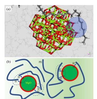
Fig. 3 (a) Structure of Model 7-25 optimized with DFTB+. The transparent blue-colored circle shows the interface part between MgO and a-PE, where four H atoms are dissociated from the PE chain and adsorbed on the MgO surface, resulting in a change into two double bonds in the PE chain and formation of four O-H covalent bonds on the MgO particle. Green, red, dark gray and white colors represent Mg, O, C and H atoms. (b) Schematic diagram summarizing the interfacial bonding mechanism.
