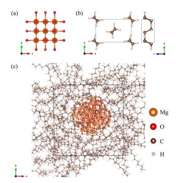
Fig. 1 Ball-and-stick view of (a) the bulk MgO unit cell in the cubic phase with a space group of  $Fm\bar{3}m$ , (b) the c-PE unit cell in the orthogonal phase with a space group of Pnma, and (c) the MgO/a-PE cubic simulation box composed of the MgO particle and surrounding a-PE chains.
