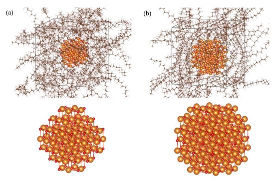
Fig. 2 Initial configurations of the MgO/a-PE composite models, (a) Model 7-25 and (b) Model 8-25, where the MgO particle radii are 7 and 8 Å respectively while the cell length of the cubic simulation box is 25 Å. The enlarged MgO particles are shown in the bottom panel.
