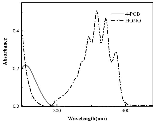
Fig. 1 UV-vis absorption spectra of 4-PCB and HONO solution.
