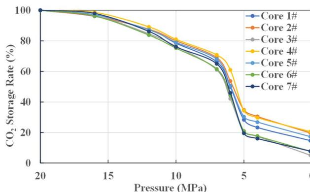
Fig. 2 Variations in the bound  $\text{CO}_2$  storage rate with pressure.
