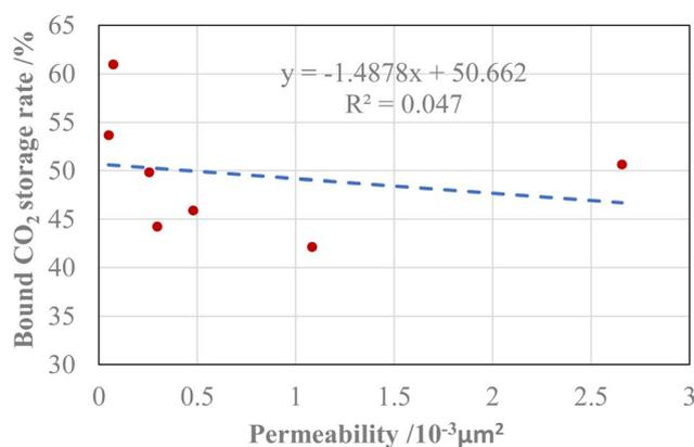
Fig. 3 The fitted relationship between bound CO<sub>2</sub> storage rate and permeability.
