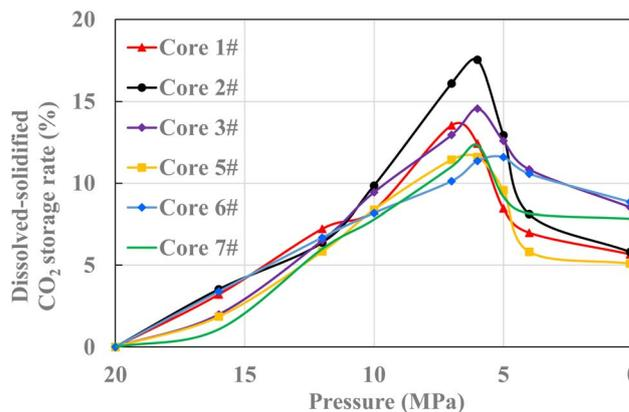
Fig. 8 The change curve of dissolved-solidified CO<sub>2</sub> storage rate with pressure.
