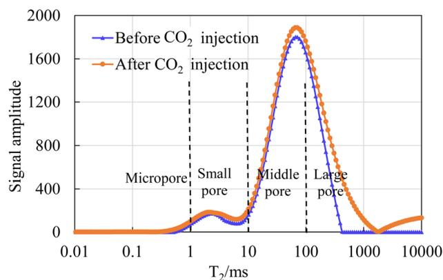
Fig. 10 The pore size distribution curve of core 2# before and after CO<sub>2</sub> injection.
