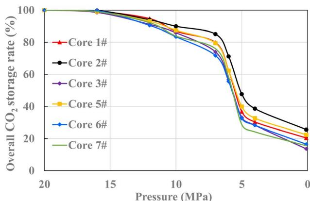
Fig. 7 The change curve of overall CO<sub>2</sub> storage rate with pressure.
