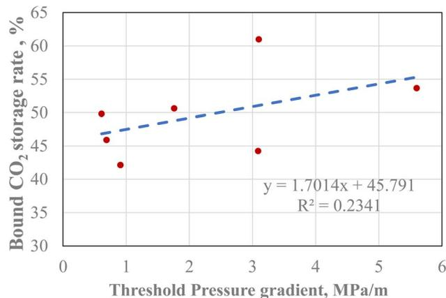
Fig. 4 The fitted relationship between bound CO<sub>2</sub> storage rate and threshold pressure gradient.
