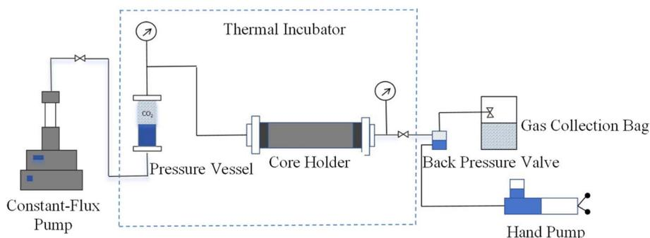
Fig. 1 Schematic diagram of the CO<sub>2</sub> storage experiment setup.
