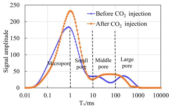
Fig. 9 The pore size distribution curve of core 1# before and after CO<sub>2</sub> injection.
