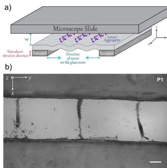
Fig. 4 HMAD in FPW-like mode. (a) Explanatory diagram of the FPW-like mode generated by the interference of Lamb waves propagating on the glass coverslip in opposite directions. Here  $w$  corresponds to the thickness of the Parafilm; (b) linear aggregates formed in a HMAD built with a Parafilm sheet P1 and two transducers at 2 MHz located in parallel, obtained at the frequency 1.872 MHz with microparticles of 4.5  $\mu\text{m}$  diameter. Scale bar  $\sim 100 \mu\text{m}$ .
