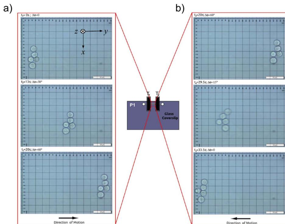
Fig. 8 Position manipulation of an aggregate of SiHa cells in HMAD P1|| in the FPW-like resonance mode due to a phase change in the acoustic wave generated by transducer 1 ( $T_1$ ). (a) Movement of the aggregate toward the right when increasing the phase difference between the transducers; and (b) movement of the aggregate toward the left when decreasing the phase difference between the transducers. Resonance was obtained with piezoelectric ceramic actuators of 2 MHz at frequency 1.873 MHz.
