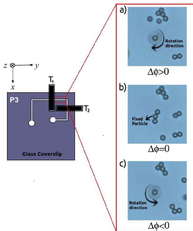
Fig. 9 Microparticle rotational motion in the HMAD P3 $\perp$  coupled with 2 MHz piezoelectric ceramic actuators at resonance frequency 1.818 MHz. (a) 4.5  $\mu\text{m}$  particles rotating clockwise around a fixed particle under a positive phase difference; (b) non-rotating particles under zero phase difference; and (c) particles rotating counterclockwise under a negative phase difference.
