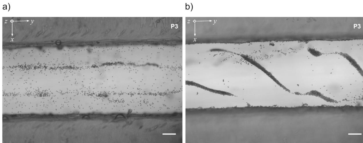
Fig. 5 Aggregates formed by microparticles of 4.5  $\mu\text{m}$  diameter in the HMADs using two transducers of 5 MHz oriented perpendicularly with the P3 geometry. (a) Two parallel linear aggregates for an experimental frequency 4.901 MHz, and (b) diagonal aggregate for an experimental frequency of 3.275 MHz. Scale bars  $\sim 100 \mu\text{m}$ .
