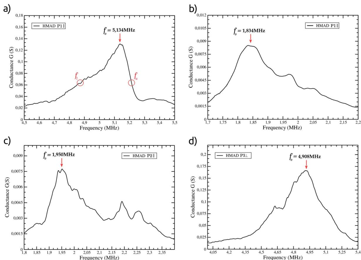
Fig. 6 Measurements of electrical conductance  $G$  of the HMADs coupled to two piezoelectric transducers. In (a and b) the electrical response (HMAD P1|| geometry) is shown, when the device is attached to two piezoelectric ceramic actuators of 5 MHz or 2 MHz respectively. (c) Electrical response of a HMAD with P2|| geometry coupled to transducers of 2 MHz; and (d) electrical characterization of a HMAD with P3⊥ geometry attached to transducers of 5 MHz.
