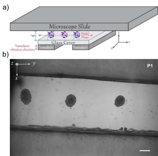
Fig. 3 HMAD in BAW-like mode. (a) Explanatory diagram of the BAW-like mode generated by the reflection of waves between the glass slide and the glass coverslip. Here  $w$  corresponds to the thickness of the Parafilm; (b) circular aggregates formed in BAW-like mode in an HMAD built with Parafilm sheet P1 and two transducers at 5 MHz located in parallel, obtained at the frequency 5.834 MHz with microparticles of 4.5  $\mu\text{m}$  diameter. Scale bar  $\sim 100 \mu\text{m}$ .
