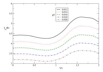
Fig. 8 In-plane RKKY interaction  $(J_{xx}(R))$  between two localized moments in undoped simple stacked bilayer graphene as a function of normalized bias voltage at fixed distance R/a = 1.0 for different normalized electron-phonon coupling strengths g/t. The temperature and magnetic field have been fixed at  $k_BT/t = 0.01$  and  $g\mu_BB/t = 0.3$ , respectively. The distance vector  $\mathbf{R} = \mathbf{R}\mathbf{R}$  is along the zigzag direction in the x-y plane, as shown in Fig. 1.
