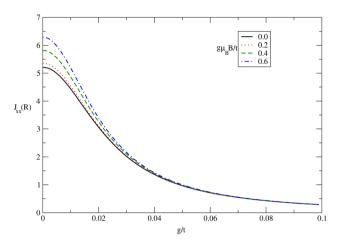
Fig. 6 In-plane RKKY interaction ( $J_{xx}(\mathbf{R})$ ) between two localized moments in undoped simple stacked bilayer graphene as a function of normalized electron-phonon coupling strength at fixed distance R/ a=1.0 for different magnetic field strengths  $g\mu_B B/t$ . The temperature and bias voltage have been fixed at  $k_BT/t = 0.01$  and V/t = 0.3, respectively. The distance vector  $\mathbf{R} = \mathbf{R}\mathbf{R}$  is along the zigzag direction in the x-y plane, as shown in Fig. 1.
