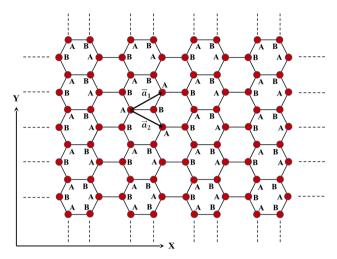
Fig. 2 Top view of AA-stacked bilayer graphene, showing the primitive lattice vectors a<sub>1</sub> and a<sub>2</sub> within a Cartesian coordinate system
