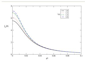
Fig. 7 In-plane RKKY interaction  $(J_{xx}(R))$  between two localized moments in undoped simple stacked bilayer graphene as a function of normalized electron-phonon coupling strength at fixed distance R/ a = 1.0 for different bias voltages V/t. The temperature and magnetic field strength have been fixed at  $k_BT/t = 0.01$  and  $g\mu_BB/t = 0.3$ , respectively. The distance vector  $\mathbf{R}=\mathbf{R}\mathbf{R}$  is along the zigzag direction in the x-y plane, as shown in Fig. 1.
