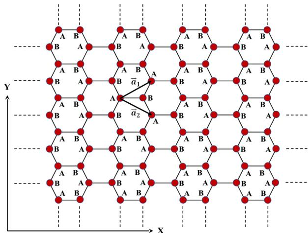
Fig. 2 Top view of AA-stacked bilayer graphene, showing the primitive lattice vectors  $\mathbf{a}_1$  and  $\mathbf{a}_2$  within a Cartesian coordinate system.
