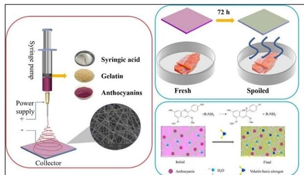
Fig. 15 Schematic representation showing the fabrication and application of the GA/PPA/SA nanofiber membrane for pork preservation and freshness monitoring.<sup>177</sup>
