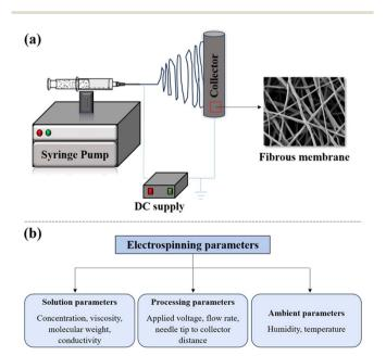
Fig. 10 (a) Schematic of a basic electrospinning setup with syringe pump, high voltage supply and collector systems. (b) Outline of various electrospinning parameters.
