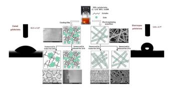
Fig. 14 Morphology of the electropsun and cast zein/gelatin films after immersion in water and ethanol for studying solvent resistance capability and their water contact angle. [Reprinted with permission from ref. 167 Copyright Elsevier 2018].
