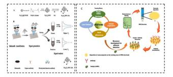
Fig. 8 (A) Preparation of  $Fe_3O_4$  NPC and  $Fe_3O_4$  NPC-SA. (B) Outline of the NMR biosensor for *Salmonella* detection in milk [reprinted with permission from ref. 112 Copyright Elsevier 2019]. (C) Electrochemical sensor based on the MoS<sub>2</sub>/UiO-66-NH<sub>2</sub> composite for AFM1 detection [Copyright © 2022, American Chemical Society].
