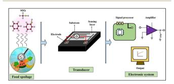
Fig. 7 Schematic depicting the gas sensing process in food quality monitoring.
