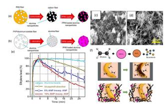
Fig. 2 Production of ANP-incorporated (a) CNFs and (b) ANFs followed by PPM casting. SEM images of ANP-incorporated (c) carbon nanofibers and (d) alumina nanofibers. (e) Ethylene absorption capacity for various absorbers. (f) Electrospun nanofiber membranes as ethylene scavengers.<sup>27</sup>. [Copyright © 2018, American Chemical Society].
