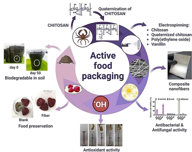
Fig. 17 Quaternized chitosan/vanillin-based nanofiber membrane as an active food packaging material [reprinted with permission from ref. 214 Copyright 2023 Elsevier].
