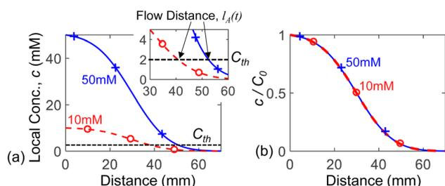
Fig. 7 (a) Numerically simulated spatial profile of concentration through the paper-channel in IHS setup shown for 10 mM and 50 mM source concentration ( $C_0$ ) at  $t = 1200$  s. The threshold  $C_{th}$  marks the flow distance  $l_A$  – see the zoomed-in plot in the inset. (b) The same plots are shown after normalization to respective source concentrations  $C_0$ .
