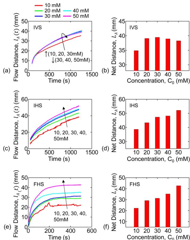
Fig. 3 Analyte flow distances through the paper-channel extracted from the experiments are shown for various concentrations. Continuous analyte flow distance ( $l_A(t)$ ) versus time for IVS, IHS, and FHS are shown in (a, c and e). Also, the end-of-experiment net flow distance versus concentration for IVS, IHS, and FHS are summarized in (b, d and f).
