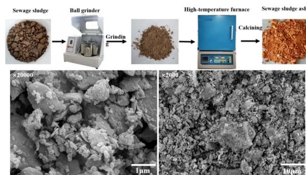
Fig. 1 Manufacturing process and microtopography of SSA.
