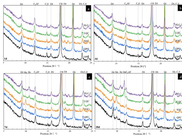
Fig. 5 XRD patterns of cement paste at various curing times: (a) 1 day, (b) 3 days, (c) 7 days, and (d) 28 days. Notes: Ett-ettringite, Ms-monosulfate, CH-portlandite, Hc-hemicarboaluminate, Mc-mono-carboaluminate, and Qz-quartz.
