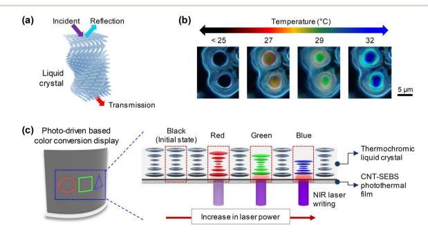
Fig. 1 Implementation of a color-conversion display based on light irradiation. (a) Schematic showing the structure of the thermochromic liquid crystals (TLCs). (b) Photographs showing the temperature-related color change. (c) Schematic showing the operation of a color-conversion display based on light irradiation with a near-infrared (NIR) laser writing on a substrate composed of TLC and carbon nanotube-styrene-ethylene-styrene (CNT-SEBS).
