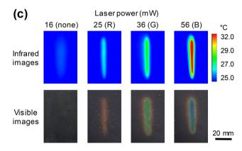
Fig. 3 Heat-generation characteristics of a color-conversion display with different NIR laser irradiation conditions. (a) Surface temperature of the display at different laser powers (20, 25, 31, 36, 39, and 56 mW). (b) RGB color expression of the display (R/G/B = 25/36/56 mW). (c) Infrared and visible images showing the surface temperature and color change of the TLC layer at different NIR laser powers.
