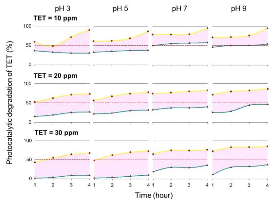
Fig. 4 Photodegradation of tetracycline (TET) by TiO<sub>2</sub>-Aq/EC material at various environmental pH and initial antibiotics concentrations.
