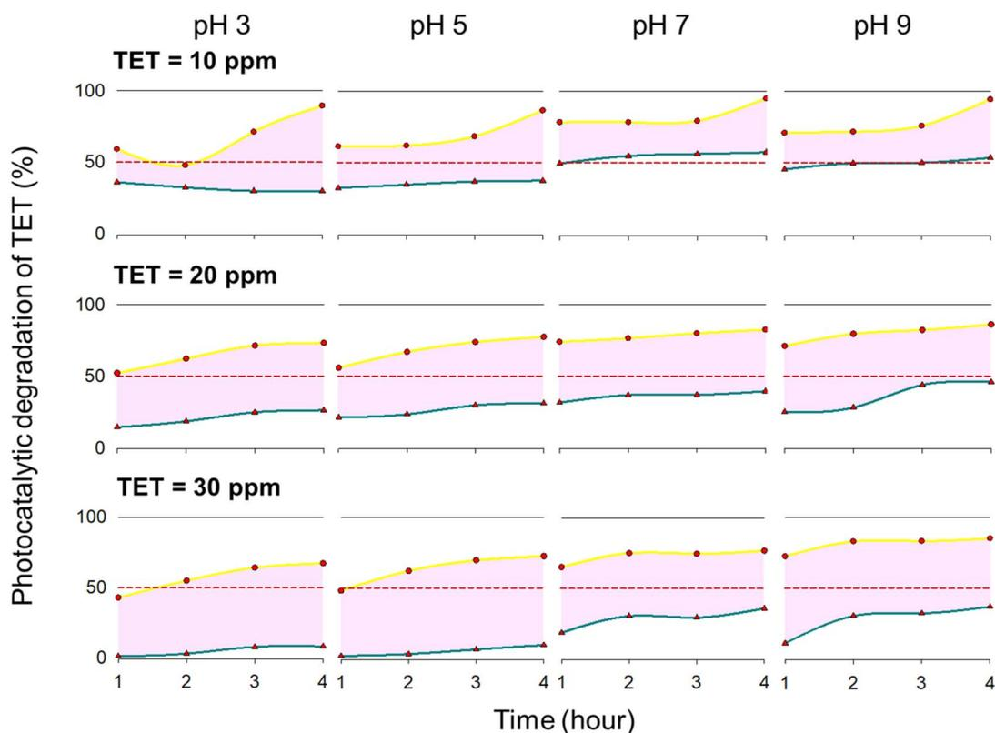
Fig. 4 Photodegradation of tetracycline (TET) by TiO<sub>2</sub>-Ag/EC material at various environmental pH and initial antibiotic concentrations.
