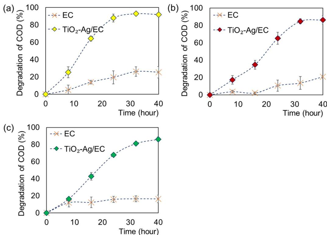
Fig. 8 Dependence of the COD removal activity of TiO<sub>2</sub>-Ag/EC on initial COD concentrations: 25 mg L<sup>-1</sup> (a), 50 mg L<sup>-1</sup> (b), and 100 mg L<sup>-1</sup> (c).
