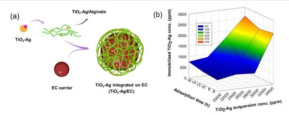
Fig. 1 Integration mechanism of  $TiO_2$ -Ag onto an expanded clay carrier (a) and impact of integration time and concentration on the immobilization of  $TiO_2$ -Ag on the EC carrier (b).
