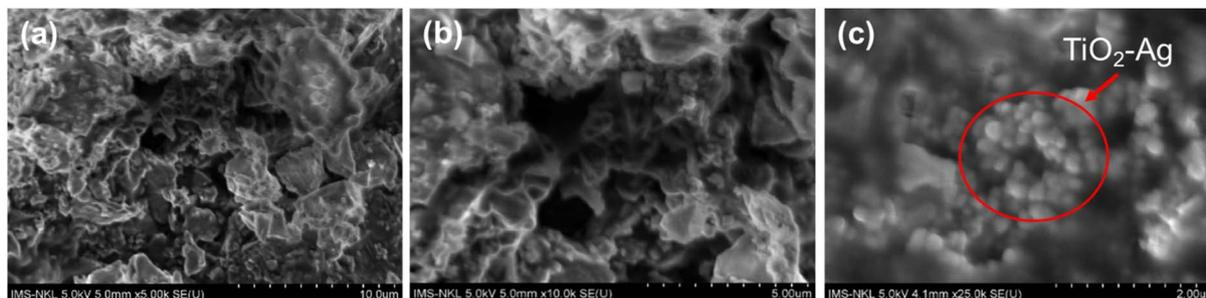
Fig. 2 FESEM images of TiO<sub>2</sub>-Ag nanoparticles integrated on EC materials at magnifications of 5 k (a), 10 k (b), and 25 k (c).
