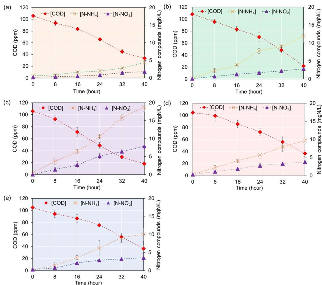
Fig. 9 Effects of various concentrations of TiO<sub>2</sub>-Ag/EC additions: 0.5% (a), 1% (b), 2.5% (c), 5% (d), and 7.5% (e) w/v on COD removal efficiency.
