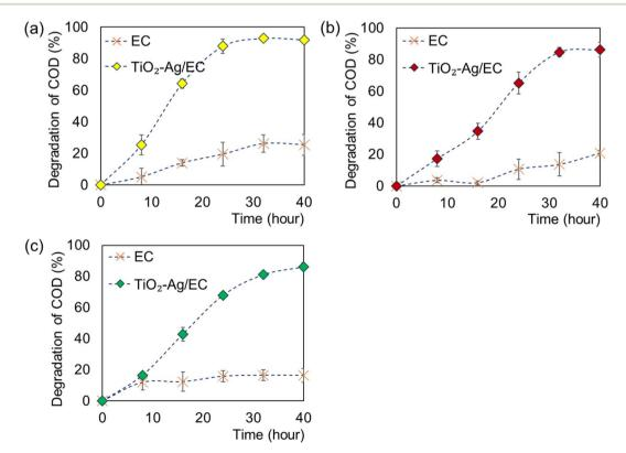
Fig. 8 Dependence of the COD removal activity of  $TiO_2$ -Aq/EC on initial COD concentrations: 25 mg  $L^{-1}$  (a), 50 mg  $L^{-1}$  (b), and 100 mg  $L^{-1}$  (c).
