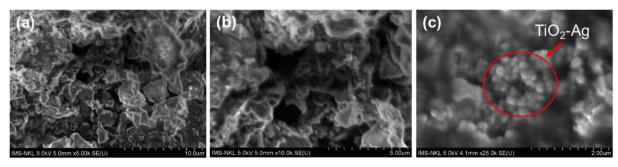
Fig. 2 FESEM images of TiO<sub>2</sub>-Aq nanoparticles integrated on EC materials at magnifications of 5 k (a), 10 k (b), and 25 k (c).
