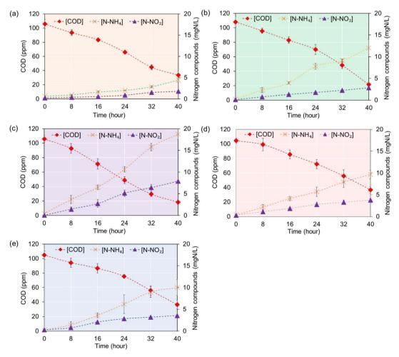
Fig. 9 Effects of various concentrations of TiO<sub>2</sub>-Aq/EC additions: 0.5% (a), 1% (b), 2.5% (c), 5% (d), and 7.5% (e) w/v on COD removal efficiency.
