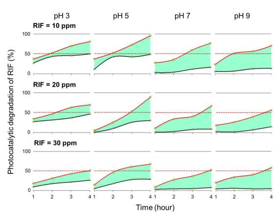
Photodegradation of rifampicin (RIF) by TiO<sub>2</sub>-Ag/EC material at various environmental pH and initial antibiotics concentrations.
