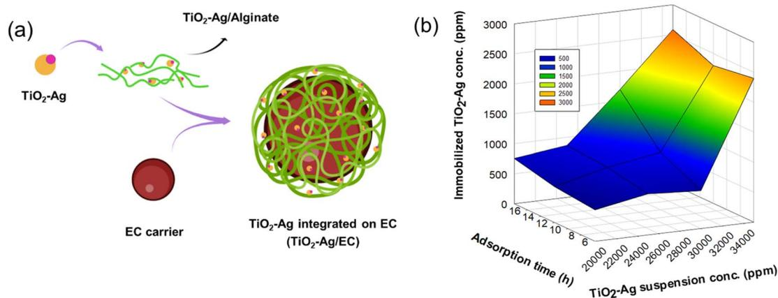
Fig. 1 Integration mechanism of  $\text{TiO}_2\text{-Ag}$  onto an expanded clay carrier (a) and impact of integration time and concentration on the immobilization of  $\text{TiO}_2\text{-Ag}$  on the EC carrier (b).
