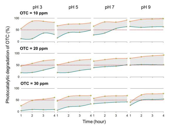
Fig. 5 Photodegradation of oxytetracycline (OTC) by TiO<sub>2</sub>-Aq/EC material at various environmental pH and initial antibiotics concentrations.
