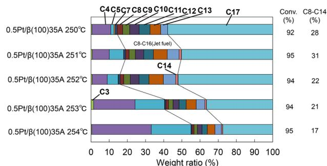
Fig. 5 Carbon number distribution of products in hydrocracking of *n*-heptadecane using pre-reduced 0.5Pt/β(100)35A. Transfer order in reaction temp.: 260 → 250 → 251 → 252 → 253 → 254 °C. H<sub>2</sub> pressure 0.5 MPa, gas flow rate 300 cm<sup>3</sup> min<sup>-1</sup>, WHSV 2.3 h<sup>-1</sup>, catalyst 2.0 g.
