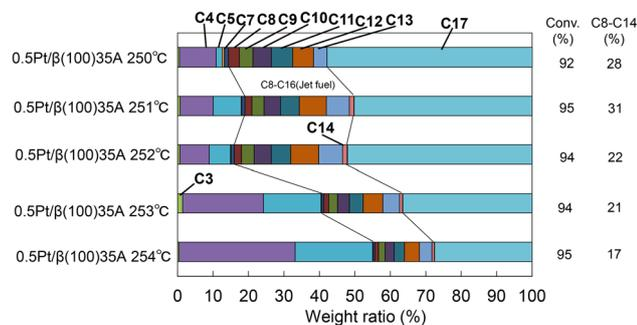
Fig. 5 Carbon number distribution of products in hydrocracking of *n*-heptadecane using pre-reduced 0.5Pt/β(100)35A. Transfer order in reaction temp.: 260 → 250 → 251 → 252 → 253 → 254 °C. H<sub>2</sub> pressure 0.5 MPa, gas flow rate 300 cm<sup>3</sup> min<sup>-1</sup>, WHSV 2.3 h<sup>-1</sup>, catalyst 2.0 g.
