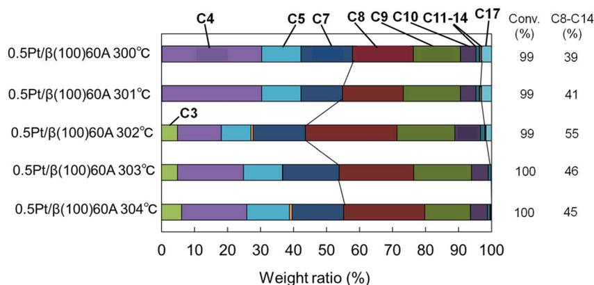
Fig. 3 Carbon number distribution of products in the fourth hydrocracking run of *n*-heptadecane using pre-reduced 0.5Pt/β(100)60A. Transfer order in reaction temp.: 310 → 308 → 306 → 304 → 302 → 300 °C. H<sub>2</sub> pressure 0.5 MPa, gas flow rate 300 cm<sup>3</sup> min<sup>-1</sup>, WHSV 2.3 h<sup>-1</sup>, catalyst 2.0 g.
