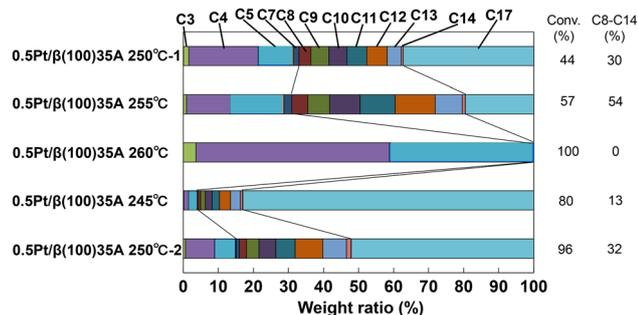
Fig. 4 Carbon number distribution of products in hydrocracking of *n*-heptadecane using pre-reduced 0.5Pt/β(100)35A. Transfer order in reaction temp.: 250 → 255 → 260 → 245 → 250 °C. H<sub>2</sub> pressure 0.5 MPa, gas flow rate 300 cm<sup>3</sup> min<sup>-1</sup>, WHSV 2.3 h<sup>-1</sup>, catalyst 2.0 g.
