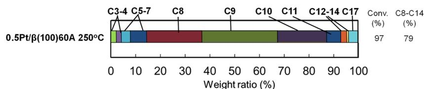
Fig. 1 Carbon number distribution of products in hydrocracking of *n*-heptadecane using 0.5Pt/ $\beta$ (100)60A without pre-reduction  $\text{H}_2$  pressure 0.5 MPa, gas flow rate 300  $\text{cm}^3 \text{min}^{-1}$ , WHSV 2.3  $\text{h}^{-1}$ , catalyst 2.0 g.
