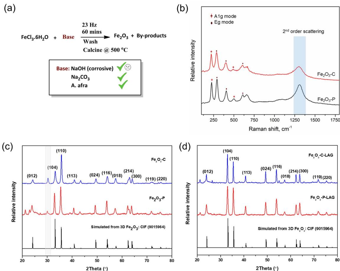
Fig. 1 (a) Chemical reactions of  $\text{Fe}_2\text{O}_3$  nanoparticles using NaOH,  $\text{Na}_2\text{CO}_3$  and plant material (*A. afra*) as a base. (b) Raman spectra of  $\text{Fe}_2\text{O}_3\text{-C/P}$  nanoparticles. (c) XRD pattern of neat  $\text{Fe}_2\text{O}_3\text{-C/P}$ , and (d) XRD pattern of LAG  $\text{Fe}_2\text{O}_3\text{-C/P}$  nanoparticles. LAG = Liquid Assisted Grinding.
