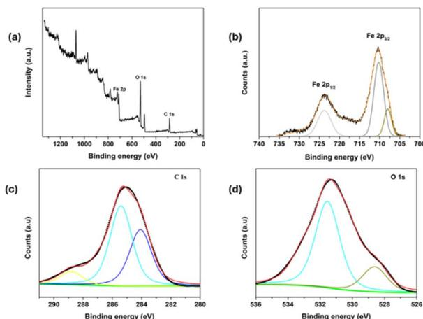
Fig. 3 XPS spectra of (a) XPS survey scan, (b) Fe 2p level, (c) C 1s level, and (d) O 1s level, of Fe<sub>2</sub>O<sub>3</sub>-C nanoparticles.
