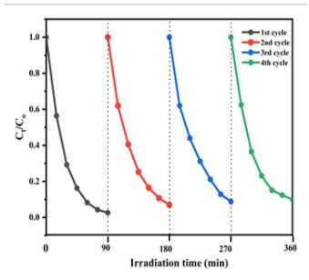
Fig. 14  $C_{t/}C_{o}$  versus time curves for the removal of CV dye over CA-N/ GO4 for various cycles.
