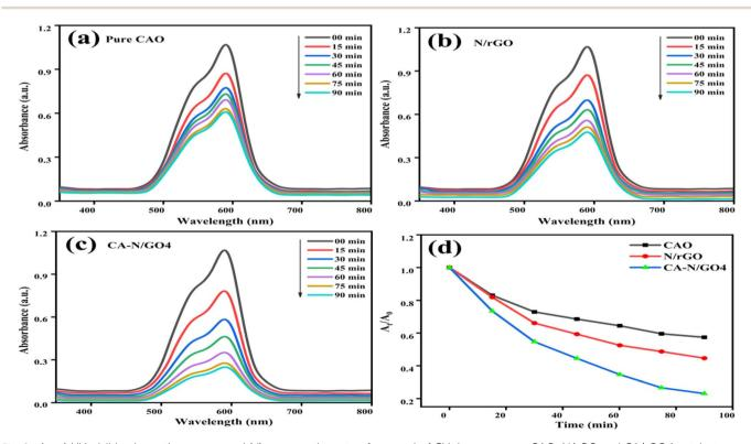
(a-c) UV-visible absorption curves and (d) comparative rate of removal of CV dye over pure CAO, N/rGO and CA/rGO4 catalysts.
