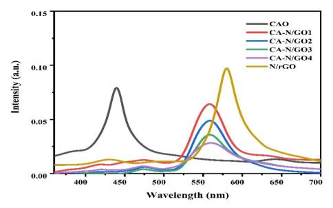
Fig. 6 PL emission spectra of pure CAO, N/rGO and CA-N/rGO nanohybrids recorded at 300 K.
