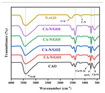
Fig. 4 FTIR spectra of pure CAO, N/rGO and CA-N/GO(1-4) nanohybrids, showing characteristic stretching and bending vibrations.
