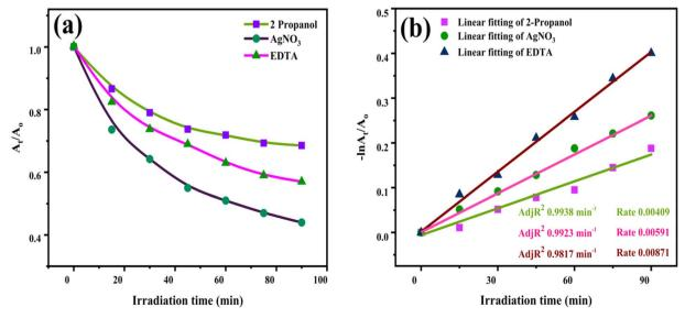
Fig. 12  $A_t/A_0$  curves (a) and (b) rate constant of scavengers for the removal of CV dye over CA-N/GO4 catalyst.
