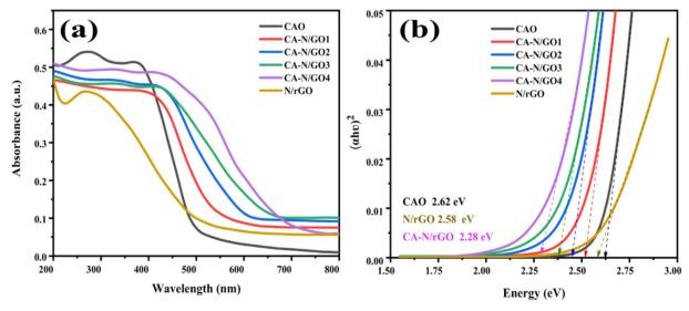
Fig. 7 (a) UV-visible absorption spectra and (b) Tauc's plot of CuAl<sub>2</sub>O<sub>4</sub>, N/rGO and CA-N/GO(1-4) nanohybrids
