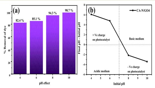
Fig. 11 (a) Effect of pH on % removal of CV dye over CA-N/GO4 photocatalyst under solar irradiation and (b) zero-point charge of CA-N/GO4.
