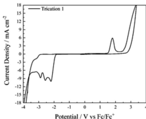
Fig. 4 Cyclic voltammogram of the Tf<sub>2</sub>N<sup>−</sup> salt of 1. Scans were conducted at 50 mV s<sup>−1</sup> from V<sub>ocp</sub>, first negative, then positive. The three sequential one-electron reduction steps are clearly apparent.
