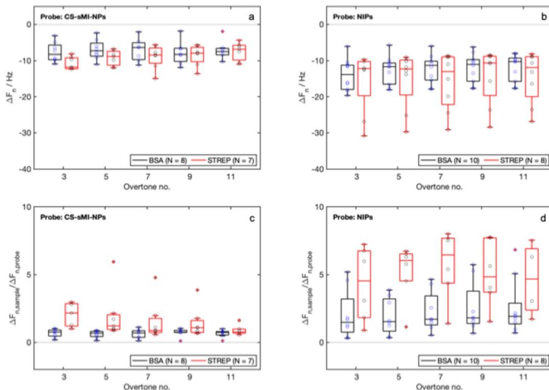
Fig. 7 QCM-D experiments, detection of the samples: (a) and (b)  $\Delta F_n$  measured for CS-sMI-NPs and NIPs after the detection of the reference protein (STREP, specific signal) and the control protein (BSA, nonspecific signal), (c) and (d) normalized  $\Delta F_n$  in respect to the values of  $\Delta F_n$  measured for probe immobilization for CS-sMI-NPs and NIPs.  $N$  indicates the number of tested sensors.
