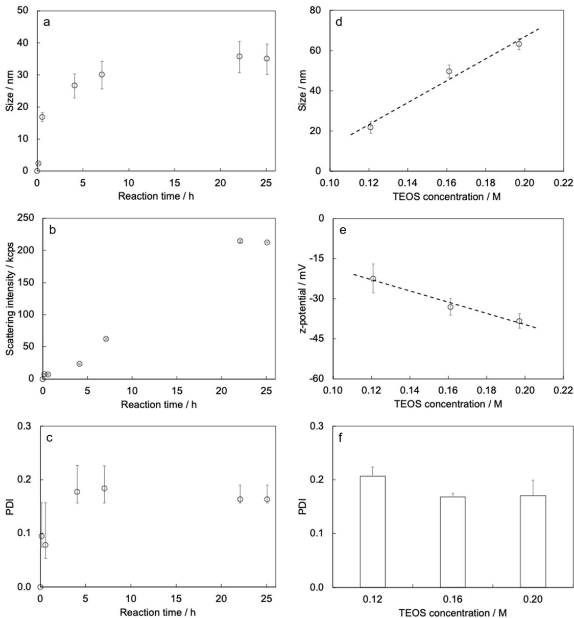
Fig. 2 Preliminary synthesis and core characterization: (a)–(c) size, scattering intensity and PDI respectively, measured during nanoparticle growth, (d)–(f) size, z-potential and PDI respectively, measured in the screening syntheses to determine the preferred TEOS concentration. In growth kinetics plots, three samples were withdrawn from the reactive mass and measured, thus reported error bars represent the range max/min.
