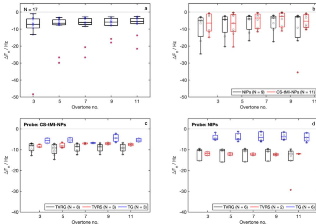
Fig. 8 QCM-D results related to the case study: (a)  $\Delta F_n$  measured after the adlayer formation; (b)  $\Delta F_n$  measured after the immobilization of the CS-tMI-NPs and NIPs; (c) and (d)  $\Delta F_n$  measured after the detection of three samples, TVRG (specific), TVRS (competitive) and TG (nonspecific) for CS-tMI-NPs and NIPs.  $N$  indicates the number of tested sensors.
