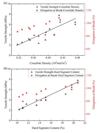
Correlation of mechanical properties with (a) crosslink density and (b) hard segment content in elastomers prepared in the BBD experiment of elongation at break.
