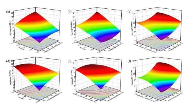
Fig. 4 Three-dimensional response surface plots of the effect of process parameters on tensile strength of polyurethane elastomers: (a) R-value and chain extension coefficient (b) R-value and curing temperature (c) chain extension coefficient and curing temperature (d) R-value and crosslinking coefficient (e) chain extension coefficient and crosslinking coefficient (f) crosslinking coefficient and curing temperature.
