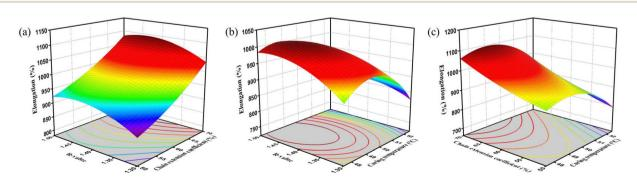
Fig. 6 Three-dimensional response surface plots of the effect of process parameters on elongation at break of polyurethane elastomers: (a) *R*-value and chain extension coefficient (b) *R*-value and curing temperature (c) chain extension coefficient and curing temperature.
