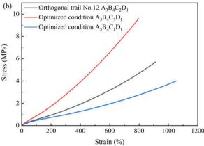
Fig. 2 Validation experiment results of the optimum conditions for maximum tensile strength (a) and maximum elongation at break (b).
