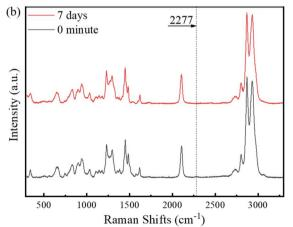
Fig. 1 FTIR (a) and Raman (b) spectra of the samples with reaction time of 0 min and 7 days.
