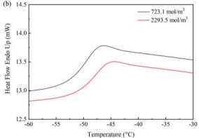
Fig. 7 Relationship of crosslink density and mechanical properties of elastomers prepared in the BBD experiment of tensile strength (a) and the DSC curves of the elastomers with the lowest and highest crosslink densities (b)
