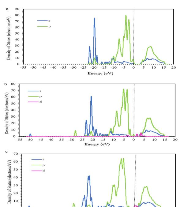
Fig. 2 Density of states (DOS) of (a) SAPO-18, (b) Zr-ZOH (Zr in 8MR), and (c) Zr-ZH (Zr in 6MR), with the local structures inserted. The vertical lines represent the position of the Fermi level
