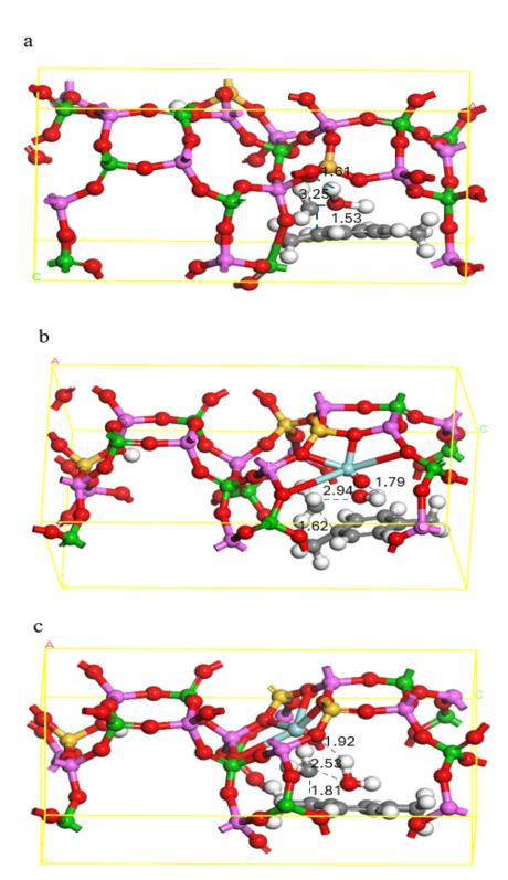
Fig. 4 Transition state (TS1-2) structures of (a) SAPO-18, (b) Zr-ZOH, and (c) Zr-ZH.
