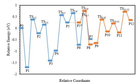
Fig. 7 Energy profile of the PX pathway in the side-chain hydrocarbon pool mechanism on Zr-ZH
