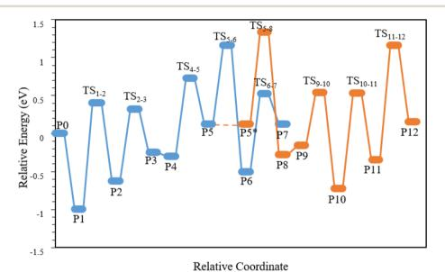
Fig. 5 Energy profile of the PX pathway in the side-chain hydrocarbon pool mechanism on SAPO-18.
