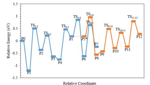
Fig. 6 Energy profile of the PX pathway in the side-chain hydrocarbon pool mechanism on Zr-ZOH.
