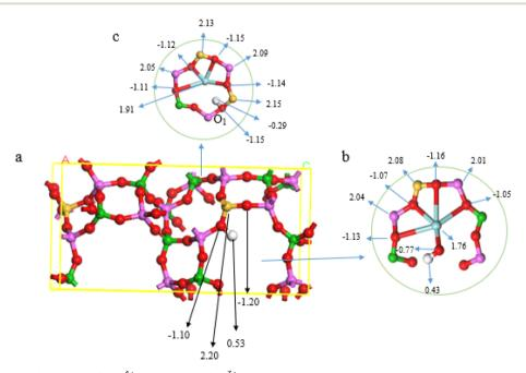
Fig. 1 Local structures for (a) SAPO-18, (b) Zr<sup>4+</sup> in 8MR, and (c) Zr<sup>3+</sup> in 6MR. Mulliken partial charges are labeled in the figure. Zr, O, Si, Al, P, and H atoms are represented in blue, red, yellow, magenta, green, and white, respectively.
