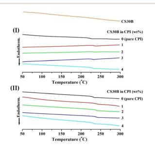
Fig. 7 DSC thermograms of CPI hybrid films containing various CS 30B contents based on (I) BAPP and (II) 6FBAPP diamine monomers.
