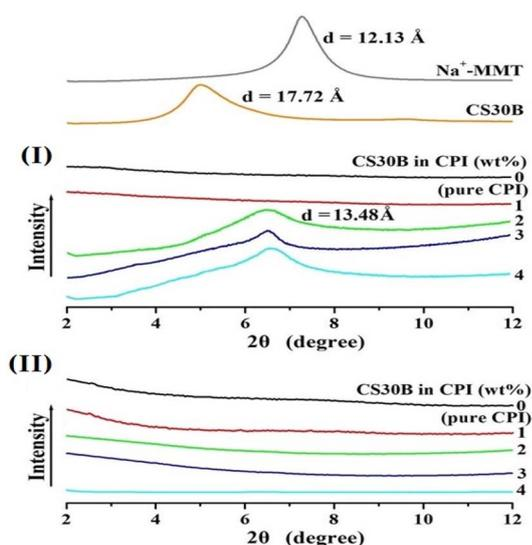
Fig. 4 XRD patterns of CPI hybrid films containing various CS30B.
