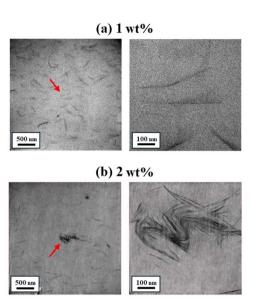
Fig. 5 TEM images of a CPI hybrid films based on BAPP diamine monomer containing different CS30B contents. (a) 1 wt% and (b) 2 wt%
