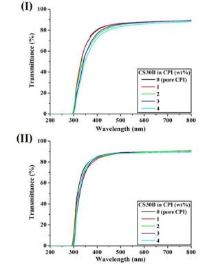
Fig. 11 UV-vis transmittance (%) of CPI hybrid films containing various CS30B contents based on (I) BAPP and (II) 6FBAPP diamine monomers.
