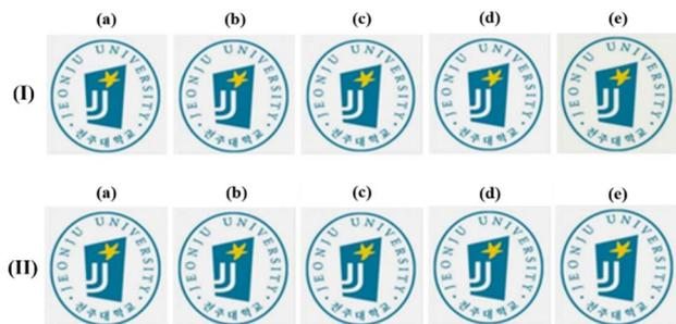
Fig. 12 Photographs of CPI hybrid films containing various CS30B contents based on (I) BAPP and (II) 6FBAPP. (a) 0 (pure CPI), (b) 1, (c) 2, (d) 3, and (e) 4 wt% CS30B.
