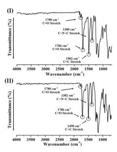
Fig. 1 FT-IR spectra of PAA and CPI.
