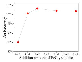
Fig. 1 Relationship between the amount of  $FeCl_3 \cdot 6H_2O$  solution added and Au recovery.
