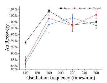
Fig. 3 Effect of oscillation frequency on Au recovery.
