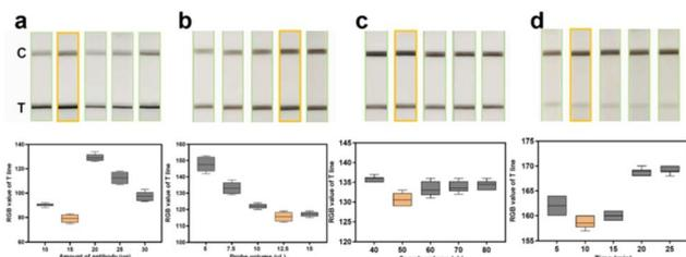
Fig. 2 Optimization of conditions for PdNP-based LFIA. (a–d) Detection results of test strips with different antibody concentrations, probe volumes, sample volumes, and incubation times between the sample and the probe.
