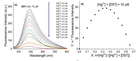
Fig. 2 (a) The fluorescence titration spectra of DST solution (10  $\mu$ M) with Hg<sup>2+</sup> at concentrations ranging from 0 to 6.5  $\mu$ M; (b) Job's plot of the interaction between Hg<sup>2+</sup> and DST (in pH 7.2 phosphate buffer, with an excitation wavelength of 368 nm, an emission wavelength of 445 nm).
