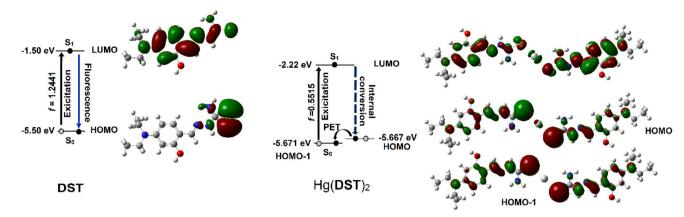
Fig. 4 Diagram illustrating the singlet electron transition processes in the excited state for DST and Hg(DST)<sub>2</sub>
