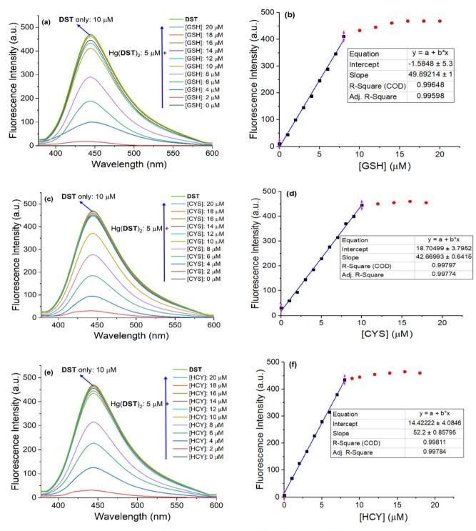
Fig. 6 Fluorescence titration results of the  $Hg(DST)_2$  complex sensor solution (5  $\mu$ M) by the thiols GSH, Cys, and Hcy (0, 1, 2, 3, 4, 5, 6, 7, 8, 9, 10, 12, 14, 16, 18, 20  $\mu$ M) in a pH 7.2 phosphate buffer, with an excitation wavelength of 368 nm and an emission wavelength of 445 nm. GSH (a and b), Cys (c and d), and Hcy (e and f).
