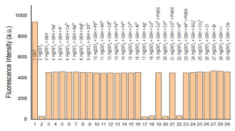
Fig. 8 Fluorescence intensity of solutions: DST (20  $\mu$ M); Hg(DST)<sub>2</sub> (10  $\mu$ M); Hg(DST)<sub>2</sub> (10  $\mu$ M) + GSH (10  $\mu$ M); Hg(DST)<sub>2</sub> (10  $\mu$ M) + GSH (10  $\mu$ M) + PHEN (1500  $\mu$ M); in a pH 7.2 phosphate buffer, with an excitation wavelength of 368 nm and an emission wavelength of 445 nm.
