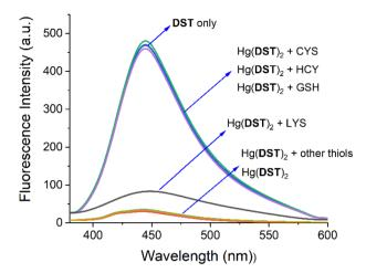
Fig. 7 Fluorescence spectra of the Hg(DST) $_2$  solution (5  $\mu$ M) upon addition of thiols GSH, Cys, and Hcy (20  $\mu$ M each), as well as amino acids Ala, Arg, Asp, Glu, Gly, His, Ile, Leu, Lys, Met, Ser, Thr, Trp, Tyr and Val (20  $\mu$ M each), in a pH 7.2 phosphate buffer, with an excitation wavelength of 368 nm and an emission wavelength of 445 nm.
