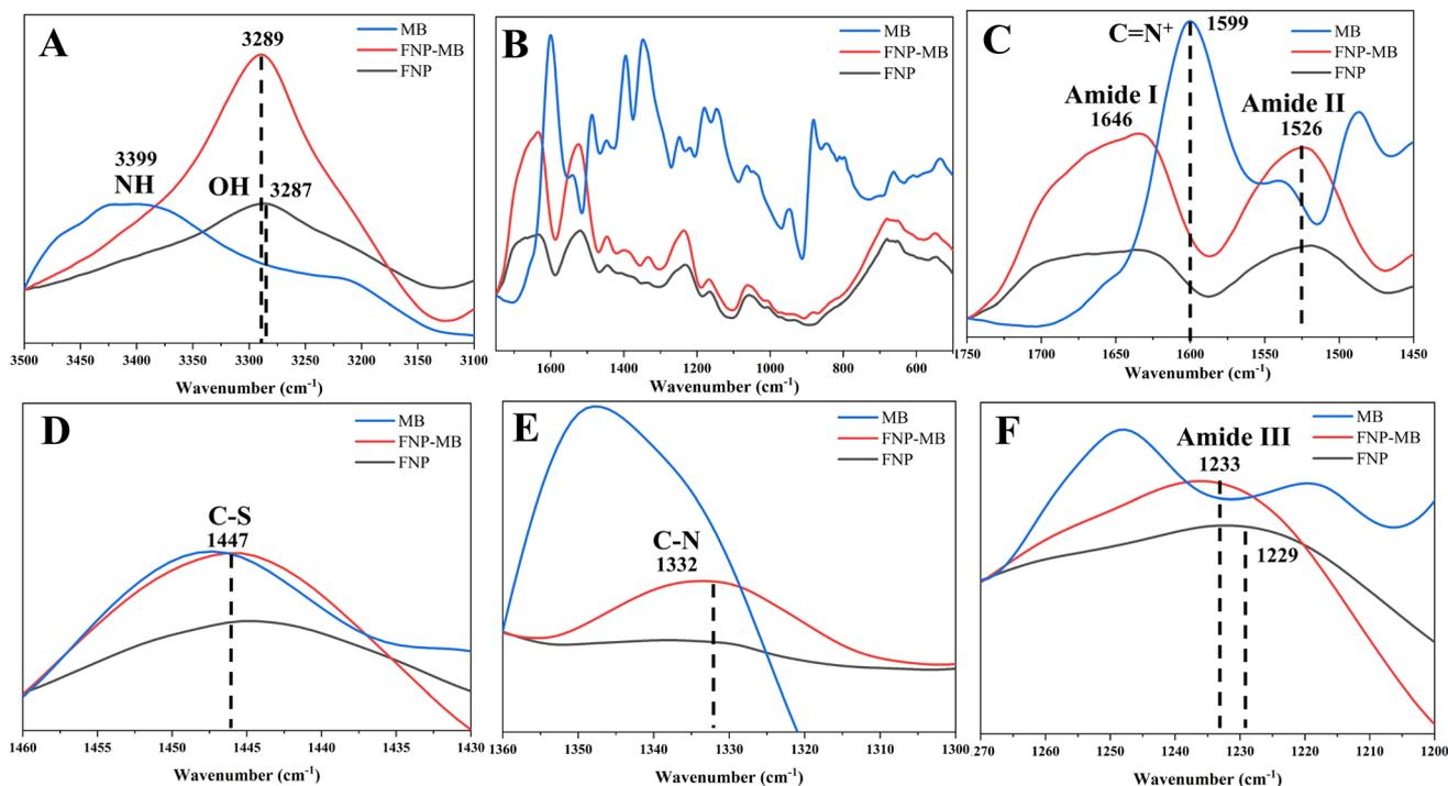
Fig. 6 FT-IR spectrum of the pure MB, FNP before adsorption, and FNP after MB adsorption (FNP-MB), at fibroin characteristic peaks of (A) 3500–3100 cm<sup>-1</sup>, (B) 1650–650 cm<sup>-1</sup>, (C) 1750–1450 cm<sup>-1</sup>, (D) 1460–1430 cm<sup>-1</sup>, (E) 1360–1300 cm<sup>-1</sup>, and (F) 1270–1200 cm<sup>-1</sup>.
