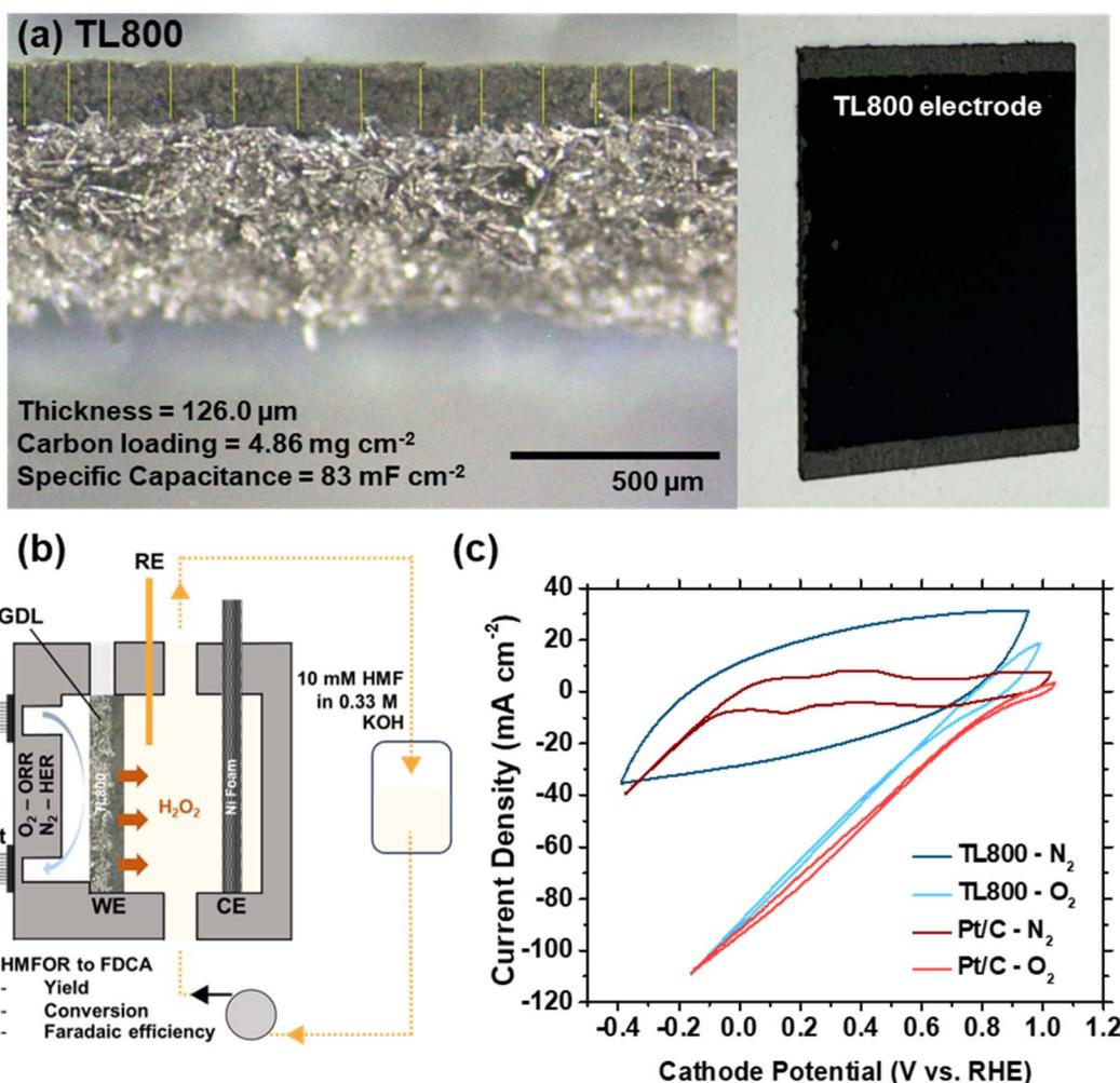
Fig. 4 (a) Optical microscopic image of TL800 electrode. (b) Schematic illustration of the GDE cell system for ORR coupled HMFOR. (c) Cyclic voltammetry of TL800 electrode and Pt/C electrode under  $\text{O}_2$  and  $\text{N}_2$  feeds.
