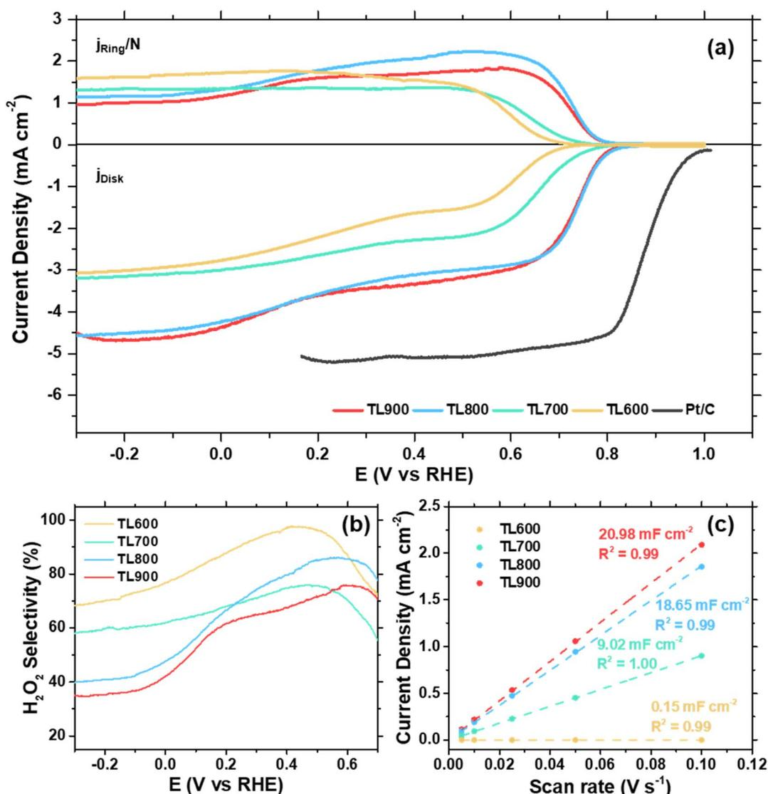
Fig. 3 (a) ORR polarization curves obtained from RRDE experiments, (b) H<sub>2</sub>O<sub>2</sub> selectivity, and (c) double-layer capacitances (*C*<sub>dl</sub>) of the tea leaf-derived carbons of different activation temperatures.
