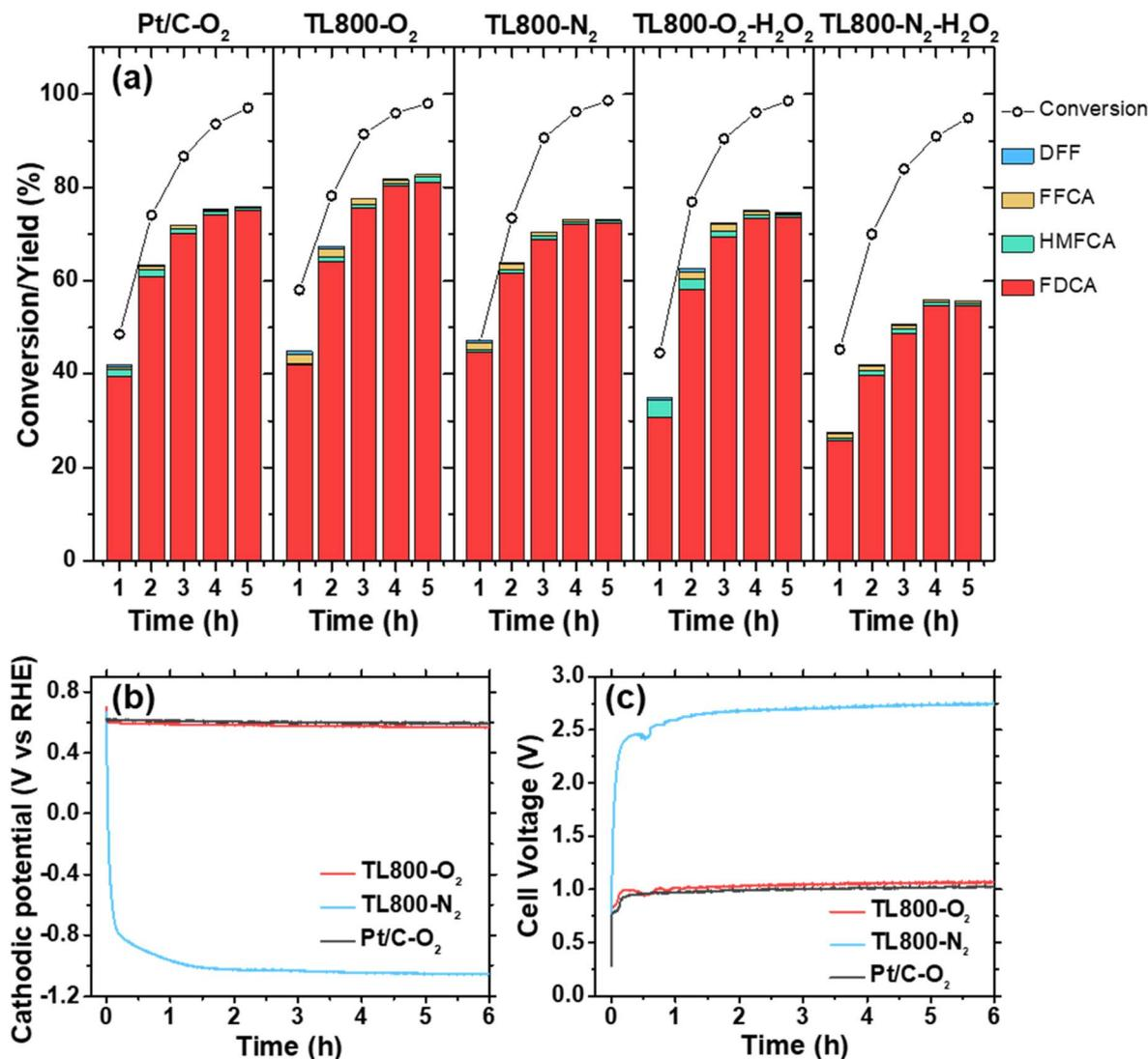
Fig. 5 (a) HMF conversion and yields of FDCA, HMFOCA, FFCA, and DFF, under different electrolysis conditions:  $O_2$ ,  $N_2$ , without and with 10 mM  $H_2O_2$  addition in the electrolyte. (b) Cathode potential and (c) cell voltage obtained during a chronopotentiometry measurement at  $10 \text{ mA cm}^{-2}$  over 6 hours.
