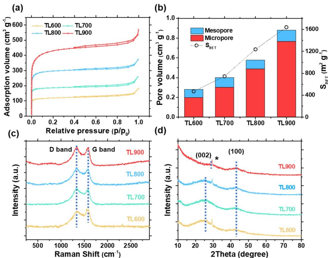
Fig. 1 (a)  $N_2$  adsorption–desorption isotherms, (b) micro–mesopore volume and  $S_{BET}$ , (c) Raman spectra, and (d) XRD patterns of the tea leaf-derived carbons obtained from different activation temperatures.
