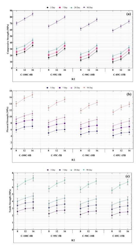
Fig. 5 Mechanical strength of GRC mixtures incorporating RBP and RCP at 7 and 28 days: (a) compressive strength, (b) flexural strength, and (c) splitting tensile strength. Results highlight the influence of recycled powder type and curing time on performance development.
