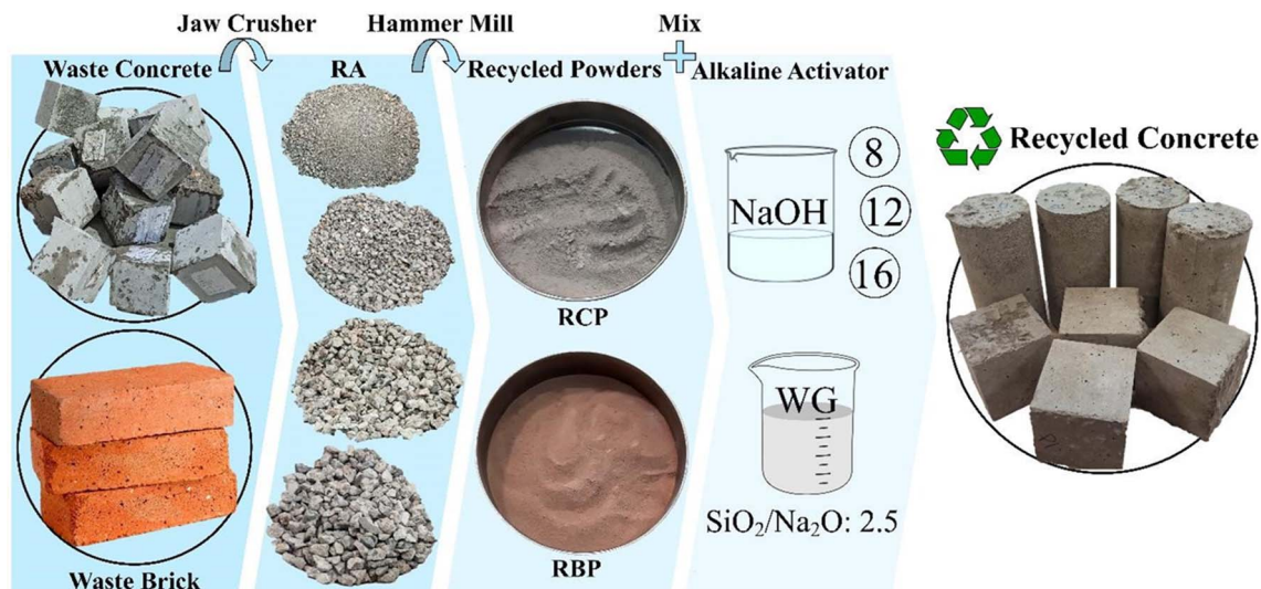
Fig. 1 Recycling process of OPC concrete into geopolymer recycled concrete (GRC), including material crushing, powder production (RCP, RBP), and mixing with alkaline activators (NaOH, WG) to form recycled concrete specimens.
