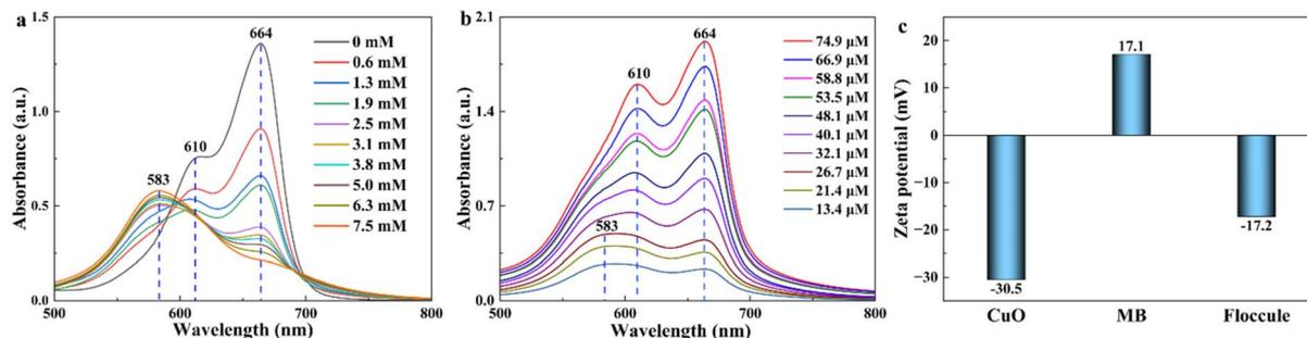
Fig. 6 In the mixed system of nano-CuO and MB: (a) absorption spectra of 26.7  $\mu\text{M}$  MB with different amounts of nano-copper oxide; (b) absorption spectra of MB with different concentrations in the presence of 2.5 mM nano-CuO; (c) zeta potential diagrams of nano-CuO, MB and the complex formed after complexation.
