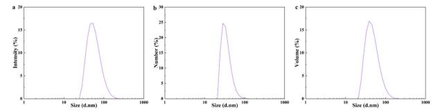
The particle size of Sample No. 6 (a) intensity-based; (b) number-based; (c) volume-based size distribution
