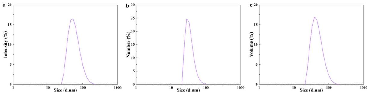
Fig. 2 The particle size of Sample No. 6 (a) intensity-based; (b) number-based; (c) volume-based size distribution.
