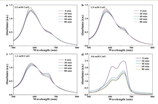
Fig. 7 Photodegradation spectra of MB with an initial concentration of 53.5  $\mu$ M under different addition amounts of nano-CuO: (a) 2.5 mM; (b) 1.9 mM; (c) 1.3 mM; (d) 0.6 mM.
