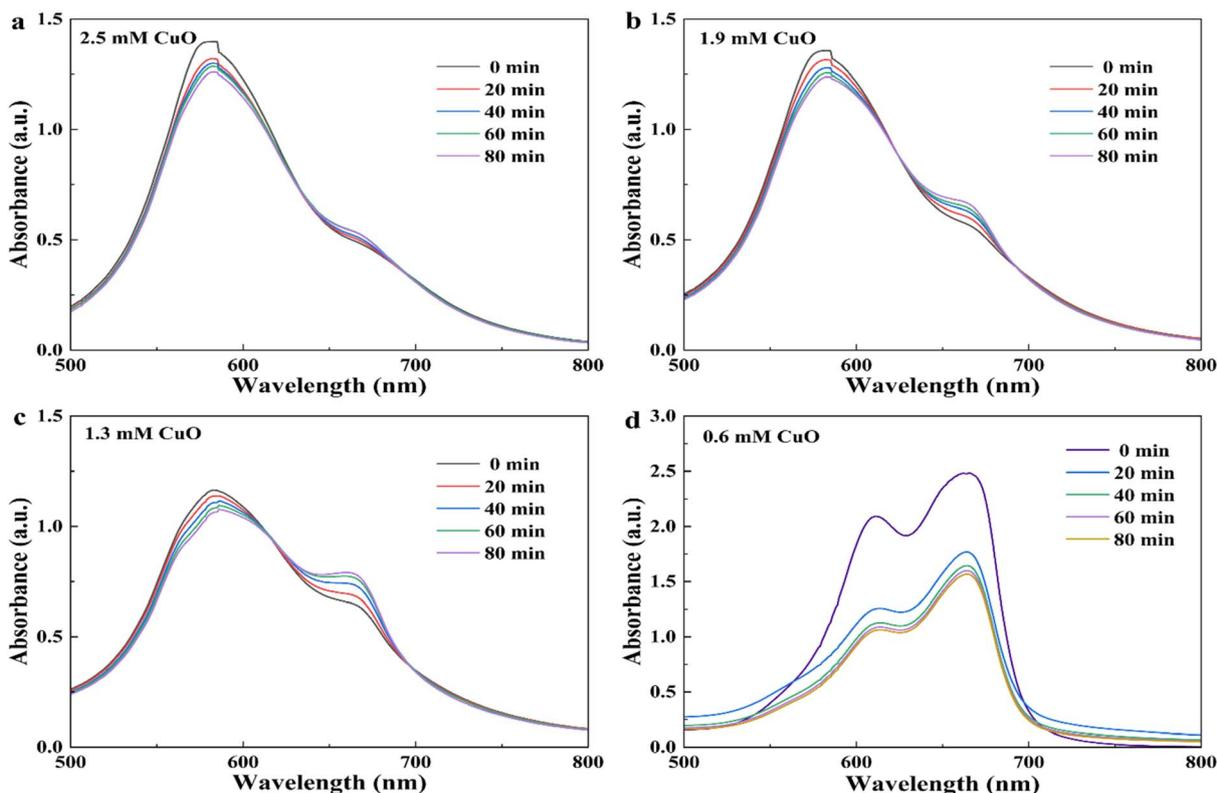
Fig. 7 Photodegradation spectra of MB with an initial concentration of 53.5  $\mu\text{M}$  under different addition amounts of nano-CuO: (a) 2.5 mM; (b) 1.9 mM; (c) 1.3 mM; (d) 0.6 mM.
