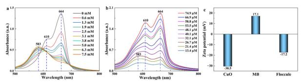
Fig. 6 In the mixed system of nano-CuO and MB: (a) absorption spectra of 26.7  $\mu$ M MB with different amounts of nano-copper oxide; (b) absorption spectra of MB with different concentrations in the presence of 2.5 mM nano-CuO; (c) zeta potential diagrams of nano-CuO, MB and the complex formed after complexation.
