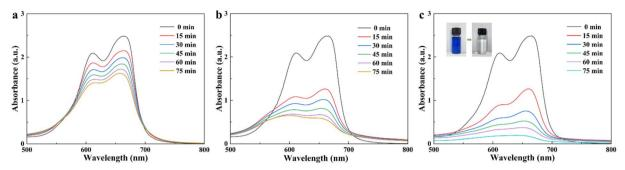
Fig. 9 Photodegradation diagram of MB (a) 0.5 mL H<sub>2</sub>O<sub>2</sub> alone; (b) 0.5 mL H<sub>2</sub>O<sub>2</sub> with 0.6 mM nano-CuO; (c) 1 mL H<sub>2</sub>O<sub>2</sub> with 0.6 mM nano-CuO.
