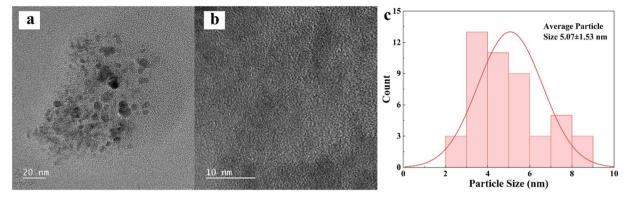
Fig. 4 (a) TEM image of Sample No. 6; (b) lattice fringe pattern of Sample No. 6; (c) particle size distribution histogram of Sample No. 6
