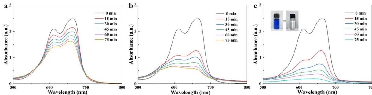
Fig. 9 Photodegradation diagram of MB (a) 0.5 mL H<sub>2</sub>O<sub>2</sub> alone; (b) 0.5 mL H<sub>2</sub>O<sub>2</sub> with 0.6 mM nano-CuO; (c) 1 mL H<sub>2</sub>O<sub>2</sub> with 0.6 mM nano-CuO.
