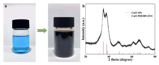
Fig. 1 (a) Optical photographs of the color change of the solution before and after the reaction (precursor on the left side, product on the right side); (b) XRD pattern of Sample No. 6.
