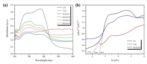
Fig. 7 (a) UV-vis DRS diffuse reflectance spectra, (b) plots of  $(\alpha h v)^{1/2}$  vs.  $h \nu$  for the band gap energy of CuS, CN and 10CuS/CN.
