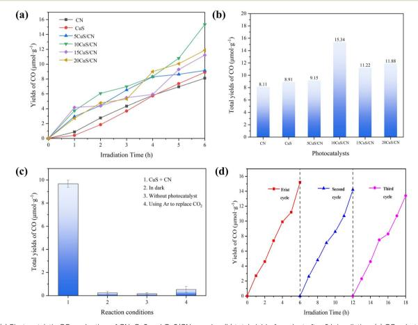
Fig. 9 (a) Photocatalytic  $CO_2$  reduction of CN, CuS and CuS/CN samples, (b) total yield of product after 6 h irradiation, (c)  $CO_2$  photocatalysis experiments under different conditions, (d) repeated experiments of 10CuS/CN sample. Reaction conditions: 50 mg photocatalyst, 100 mL deionized water, 100 kPa  $CO_2$  (99.999%) 30 min, T=25 °C, the photocatalytic time was 6 hours.
