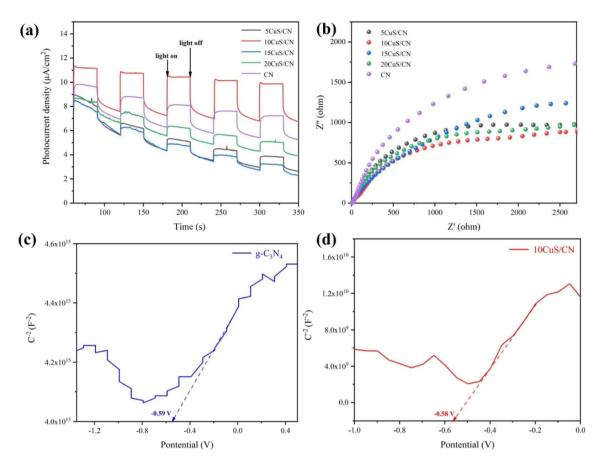
Fig. 10 (a) Photocurrent (PC), (b) electrochemical impedance spectroscopy (EIS) of CN and xCuS/CN; Mott–Schottky plots measured for (c) CN and (d) 10CuS/CN.
