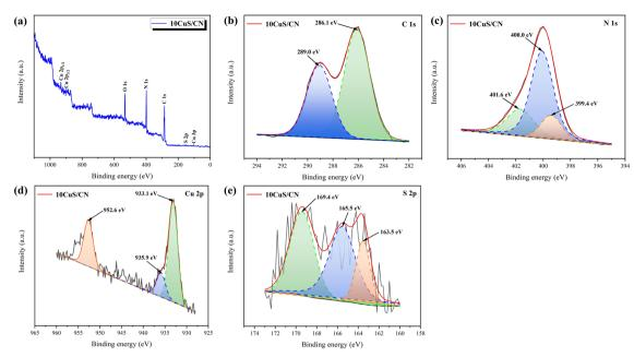
Fig. 3 (a) Full XPS spectrum of the prepared 10CuS/CN; (b) high-resolution XPS spectra of C 1s, (c) N 1s, (d) S 2p, and (e) Cu 2p.
