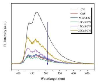
Fig. 8 Photoluminescence spectra of CuS, CN, and different wt% of CuS/CN composites.
