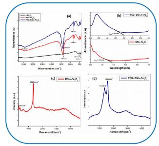
Fig. 2 FTIR spectra of (a)  $\alpha$ -Fe<sub>2</sub>O<sub>3</sub>, BN/ $\alpha$ -Fe<sub>2</sub>O<sub>3</sub>, and PEG-BN/ $\alpha$ -Fe<sub>2</sub>O<sub>3</sub>, UV-visible absorption spectra of (b) BN/ $\alpha$ -Fe<sub>2</sub>O<sub>3</sub> and PEG-BN/ $\alpha$ -Fe<sub>2</sub>O<sub>3</sub>, Raman spectra of (c) BN/ $\alpha$ -Fe<sub>2</sub>O<sub>3</sub> and (d) PEG-BN/ $\alpha$ -Fe<sub>2</sub>O<sub>3</sub>.
