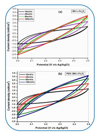
Fig. 6 Cyclic voltammetry analysis of (a)  $BN/\alpha$ -Fe<sub>2</sub>O<sub>3</sub>, (b) PEG-BN/ $\alpha$ -Fe<sub>2</sub>O<sub>3</sub> composites produced by the hydrothermal procedure.
