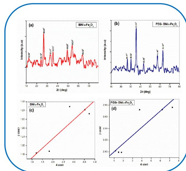
Fig. 1 XRD analysis of hydrothermal method-assisted synthesis of (a) BN/ $\alpha$ - $\text{Fe}_2\text{O}_3$  composites, (b) PEG-BN/ $\alpha$ - $\text{Fe}_2\text{O}_3$  composites. Williamson–Hall analysis plotted between  $4 \sin \theta$  against  $\beta \cos \theta$  of (c) BN/ $\alpha$ - $\text{Fe}_2\text{O}_3$  and (d) PEG-BN/ $\alpha$ - $\text{Fe}_2\text{O}_3$  produced using the hydrothermal synthesis route.
