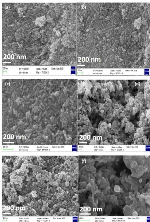
Fig. 5 SEM micrographs of (a), (b) and (c) BN/ $\alpha$ -Fe<sub>2</sub>O<sub>3</sub> and (d), (e) and (f) PEG-BN/ $\alpha$ -Fe<sub>2</sub>O<sub>3</sub> at different magnifications produced using the hydrothermal process.
