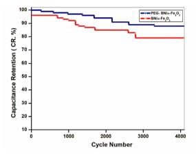
Fig. 8 Cyclic stability determination of hydrothermally prepared BN/ $\alpha$ -Fe<sub>2</sub>O<sub>3</sub> and PEG-BN/ $\alpha$ -Fe<sub>2</sub>O<sub>3</sub> composites obtained after 1st and 5000 cycles, capacitance retention (%) *versus* cycle number.
