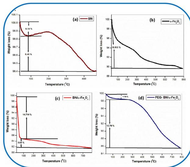
Fig. 4 TGA plot (Temperature v/s Weight loss), of (a) BN, (b)  $\alpha$ -Fe<sub>2</sub>O<sub>3</sub>, (c) BN/ $\alpha$ -Fe<sub>2</sub>O<sub>3</sub> and (d) PEG-BN/ $\alpha$ -Fe<sub>2</sub>O<sub>3</sub> composites prepared using the hydrothermal technique.
