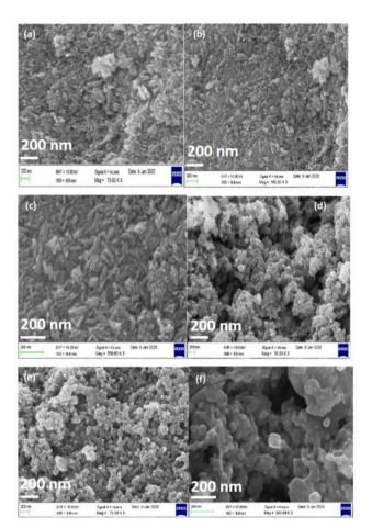
Fig. 5 SEM micrographs of (a), (b) and (c)  $BN/\alpha$ - $Fe_2O_3$  and (d). (e) and (f)  $PEG-BN/\alpha$ - $Fe_2O_3$  at different magnifications produced using the hydrothermal process.
