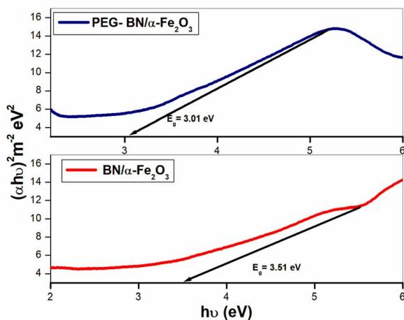
Fig. 3 Tauc plot analysis of BN/ $\alpha$ -Fe<sub>2</sub>O<sub>3</sub> and PEG-BN/ $\alpha$ -Fe<sub>2</sub>O<sub>3</sub> composites synthesized via the hydrothermal method, illustrating their optical bandgap.
