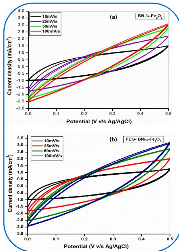
Fig. 6 Cyclic voltammetry analysis of (a) BN/ $\alpha$ -Fe<sub>2</sub>O<sub>3</sub>, (b) PEG-BN/ $\alpha$ -Fe<sub>2</sub>O<sub>3</sub> composites produced by the hydrothermal procedure.
