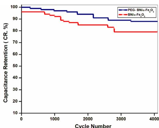
Fig. 8 Cyclic stability determination of hydrothermally prepared BN/ $\alpha$ -Fe<sub>2</sub>O<sub>3</sub> and PEG-BN/ $\alpha$ -Fe<sub>2</sub>O<sub>3</sub> composites obtained after 1st and 5000 cycles, capacitance retention (%) versus cycle number.
