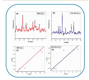
Fig. 1 XRD analysis of hydrothermal method-assisted synthesis of (a) BN/ $\alpha$ -Fe<sub>2</sub>O<sub>3</sub> composites, (b) PEG-BN/ $\alpha$ -Fe<sub>2</sub>O<sub>3</sub> composites. Williamson–Hall analysis plotted between 4 sin  $\theta$  against  $\beta$  cos  $\theta$  of (c) BN/ $\alpha$ -Fe<sub>2</sub>O<sub>3</sub> and (d) PEG-BN/ $\alpha$ -Fe<sub>2</sub>O<sub>3</sub> produced using the hydrothermal synthesis route.
