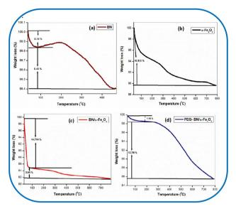
Fig. 4 TGA plot (Temperature v/s Weight loss), of (a) BN, (b) $\alpha$ -Fe<sub>2</sub>O<sub>3</sub>, (c)BN/ $\alpha$ -Fe<sub>2</sub>O<sub>3</sub>, and (d)PEG-BN/ $\alpha$ -Fe<sub>2</sub>O<sub>3</sub> composites prepared using the hydrothermal technique.
