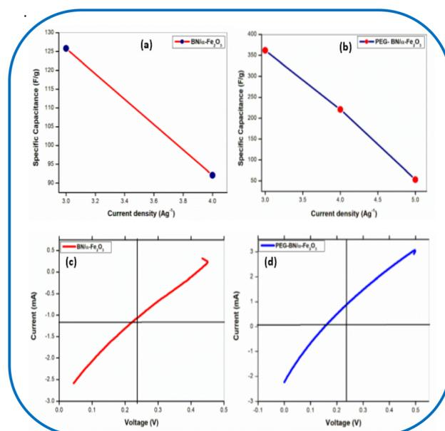
Fig. 9 Illustrates the variation of specific capacitance with an increase in current density for (a) BN/ $\alpha$ -Fe<sub>2</sub>O<sub>3</sub> and (b) PEG-BN/ $\alpha$ -Fe<sub>2</sub>O<sub>3</sub> composites produced by hydrothermal process, and the *I-V* measurements of hydrothermally synthesized (c) BN/ $\alpha$ -Fe<sub>2</sub>O<sub>3</sub> and (d) PEG-BN/ $\alpha$ -Fe<sub>2</sub>O<sub>3</sub> composites to analyze their electrical behavior.
