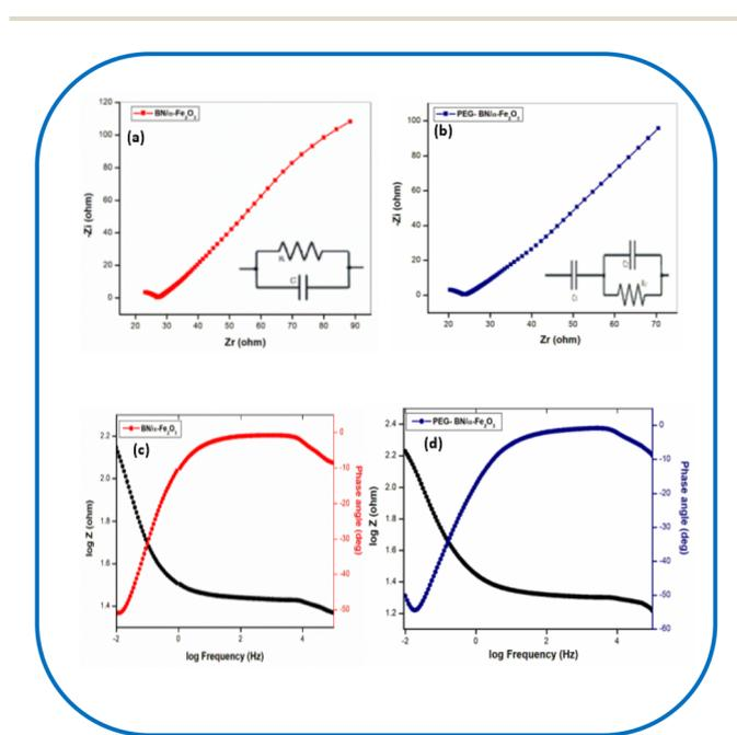
Fig. 10 Nyquist plots for (a) BN/ $\alpha$ -Fe<sub>2</sub>O<sub>3</sub> and (b) PEG-BN/ $\alpha$ -Fe<sub>2</sub>O<sub>3</sub> composites and bode plots for (c) BN/ $\alpha$ -Fe<sub>2</sub>O<sub>3</sub> and (d) PEG-BN/ $\alpha$ -Fe<sub>2</sub>O<sub>3</sub> composites synthesized *via* the hydrothermal method.
