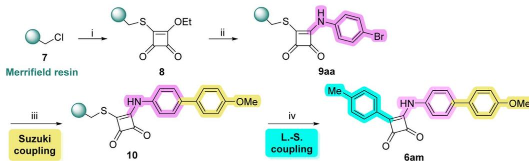
Scheme 4 Synthesis of squaramides *via* chemoselective approach. <sup>a</sup>Reagents and conditions: (i) 3-ethoxy-4-mercaptocyclobut-3-ene-1,2-dione, TEA, DMF, rt, 18 h; (ii) 4-bromoaniline, DCM, 50 °C, 18 h; (iii) 4-(methoxyphenyl)boronic acid, KOAc, PdCl<sub>2</sub>(dppf), anhydrous DMF, 60 °C, 18 h; (iv) *p*-tolylboronic acid, CuTC, TFP, Pd<sub>2</sub>(dba)<sub>3</sub>, anhydrous dioxane, 50 °C, 18 h.
