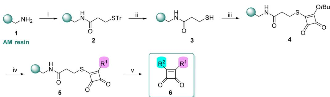
**Scheme 2** Synthesis of squaramides **6** using aminomethyl resin. <sup>a</sup>Reagents and conditions: (i) 3-(tritylthio)propionic acid, DIC, DCM/DMF (1 : 1), rt, 18 h; (ii) TFA/TES (95 : 5), rt, 1 h; (iii) 3-(*tert*-butoxy)-4-methoxycyclobut-3-ene-1,2-dione, TEA, DCM, rt, 18 h; (iv) amines (or other nucleophiles), DCM, (TEA – for Nu–H·HCl), rt, 18 h; (v) R<sup>2</sup>–B(OH)<sub>2</sub>, CuTC, TFP, Pd<sub>2</sub>(dba)<sub>3</sub>, dioxane anhydrous, 50 °C, 18 h.
