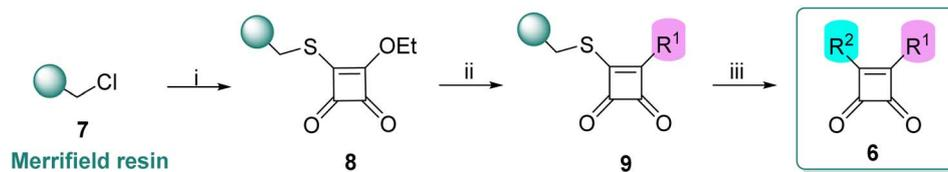
**Scheme 3** Synthesis of squaramides **6** using Merrifield resin. <sup>a</sup>Reagents and conditions: (i) 3-ethoxy-4-mercaptocyclobut-3-ene-1,2-dione, TEA, DMF, rt, 18 h; (ii) amines (or other nucleophiles), DCM, (TEA – for Nu–H·HCl), rt–50 °C, 18 h; (iii) R<sup>2</sup>–B(OH)<sub>2</sub>, CuTC, TFP, Pd<sub>2</sub>(dba)<sub>3</sub>, anhydrous dioxane, 50 °C, 18 h.
