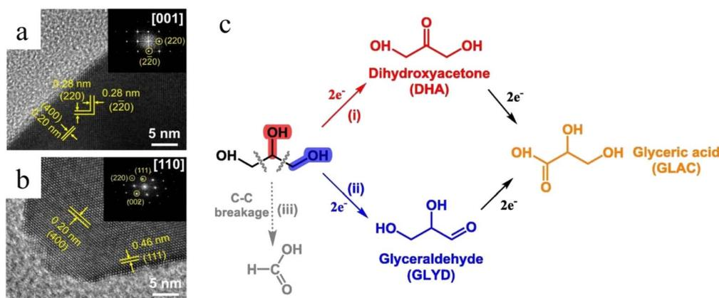
Fig. 9 HRTEM analysis of (a) C- $\text{Co}_3\text{O}_4$  and (b) O- $\text{Co}_3\text{O}_4$ .<sup>60</sup> (c) Proposed reaction pathway of the GEOR over O- $\text{Co}_3\text{O}_4$ .<sup>60</sup> Reproduced with permission from ref. 60. Copyright 2023, Elsevier.
