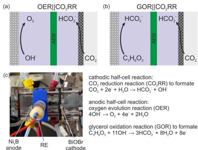
Fig. 13 Schematic representation of an OER||CO<sub>2</sub>RR reactor (a) and GOR||CO<sub>2</sub>RR paired electrolyzer (b), and picture of a used paired electrolyzer (c).<sup>70</sup> Reproduced with permission from ref. 70. Copyright 2023, Wiley-VCH.
