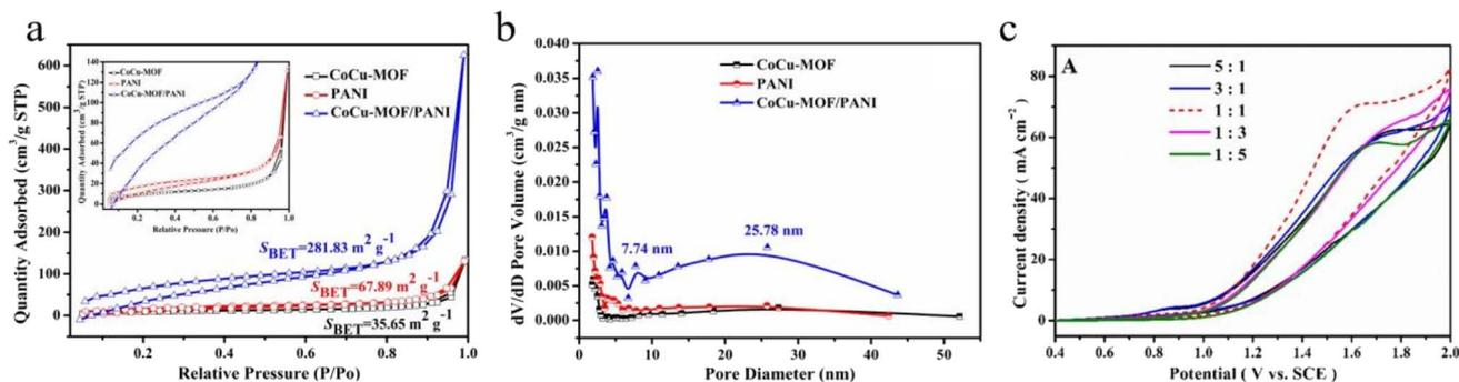
Fig. 11 (a)  $N_2$  adsorption–desorption isotherms and (inset) partially enlarged plot and (b) corresponding pore size distribution of CoCu-MOF, PANI and CoCu-MOF/PANI.<sup>64</sup> (c) CV curves of CoCu-MOF/PANI with different mass ratios in  $0.5 \text{ mol L}^{-1} \text{ KOH} + 0.5 \text{ mol L}^{-1} \text{ C}_3\text{H}_8\text{O}_3$ .<sup>64</sup> Copyright (2020), with permission from Elsevier. Reproduced with permission from ref. 64. Copyright 2020, Elsevier.
