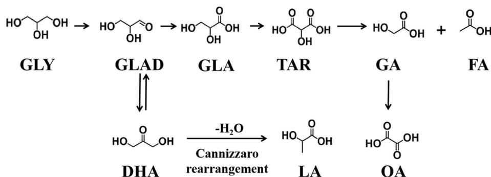
Fig. 2 Possible reaction pathways for glycerol oxidation.
