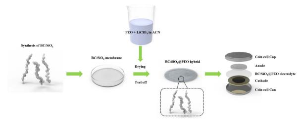
Fig. 1 Schematic diagram of BC/SiO<sub>2</sub>@PEO composite synthesis procedure.
