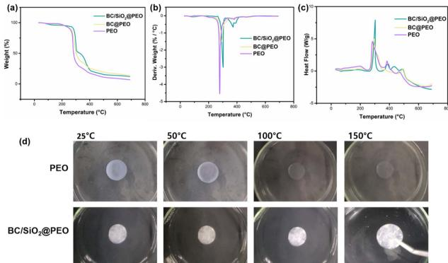
Fig. 3 (a) Thermogravimetric analysis (TGA), (b) differential thermal analysis (DTA), and (c) differential scanning calorimetry (DSC) curves of PEO, BC@PEO, and BC/SiO<sub>2</sub>@PEO solid polymer electrolytes. (d) Optical images of the electrolytes at different temperatures (25 °C, 50 °C, 100 °C, and 150 °C)
