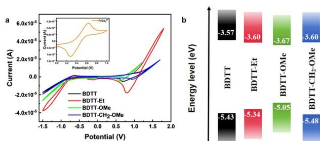
Fig. 2 (a) CV curves of the four compounds in a 0.1 mol per L acetonitrile solution, scan rate:  $20 \text{ mV s}^{-1}$ , with ferrocene/ferrocenium (Fc/Fc<sup>+</sup>) couple provided as internal standard. (b) Energy level diagrams of the four compounds.
