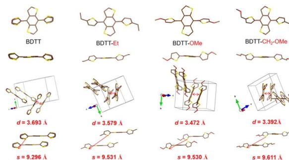
Fig. 3 Crystal structures of BDTT, BDTT-Et, BDTT-OMe and BDTT-CH<sub>2</sub>-OMe.
