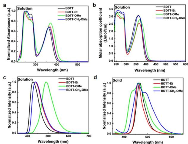
Fig. 1 (a) Normalized UV-vis absorption spectra of the four compounds in chloroform solution at a concentration of  $1 \times 10^{-5} \text{ mol L}^{-1}$ . (b) Molar absorption coefficients of the four compounds. (c) PL spectra of the four compounds in chloroform solution at a concentration of  $1 \times 10^{-5} \text{ mol L}^{-1}$ . (d) PL spectra of the four compounds in their solid states.
