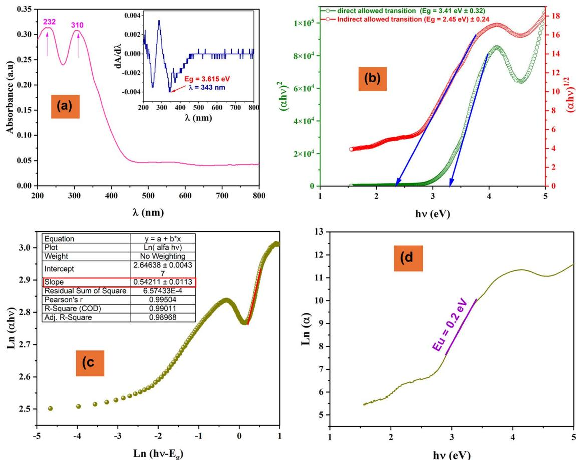
Fig. 4 (a) Absorbance as a function of wavelength for  $\text{Li}_2\text{MgZrO}_4$ , with the derivative of absorbance displayed in the inset. (b) Plot of  $(\alpha h\nu)^{1/2}$  and  $(\alpha h\nu)^2$  against  $h\nu$  for the  $\text{Li}_2\text{MgZrO}_4$  compound. (c) Evolution of  $\ln(\alpha h\nu)$  vs.  $\ln(h\nu - E_g)$  for the  $\text{Li}_2\text{MgZrO}_4$  compound. (d)  $\ln(\alpha)$  vs.  $h\nu$  plots to determine the Urbach energy  $E_U$ .
