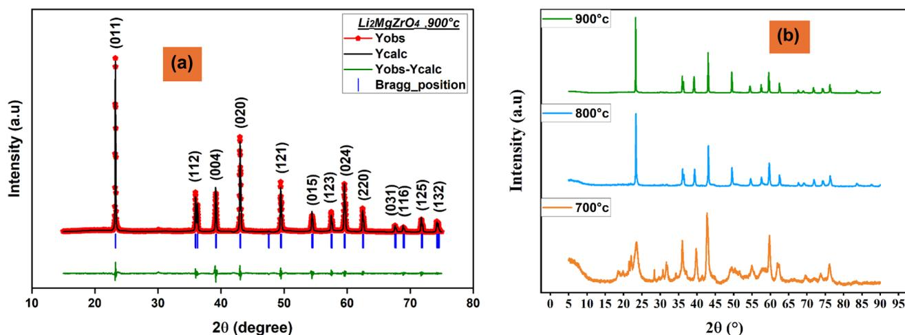
Fig. 1 (a) Rietveld refinement pattern of XRD data of  $\text{Li}_2\text{MgZrO}_4$  at room temperature, (b): XRD patterns of the sample measured at temperatures of  $700 \text{ }^\circ\text{C}$ ,  $800 \text{ }^\circ\text{C}$ , and  $900 \text{ }^\circ\text{C}$ .
