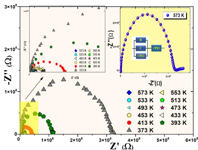
Fig. 5 Nyquist plots ( $Z''$  vs.  $Z'$ ) for  $\text{Li}_2\text{MgZrO}_4$  compound in the temperature range from 373 K to 573 K with the inset showing the equivalent circuit model used for the fitting procedure.
