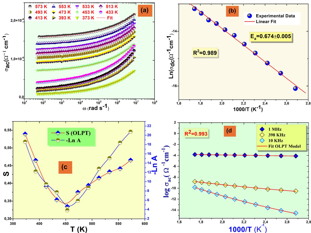
Fig. 13 (a) Electrical conductivity spectra of the studied system at various temperatures, (b) temperature dependence of the  $\sigma_{dc}$  as a function of the temperature with corresponding activation energy, (c) the temperature dependence of the frequency exponent  $S$ , (d) variation of AC conductivity versus  $1000/T$  OLPT model.
