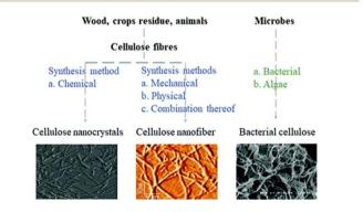
Fig. 3 Morphology of CNCs, CNFs, and BNC. Reproduced from ref. 47 with permission from the Royal Society of Chemistry.
