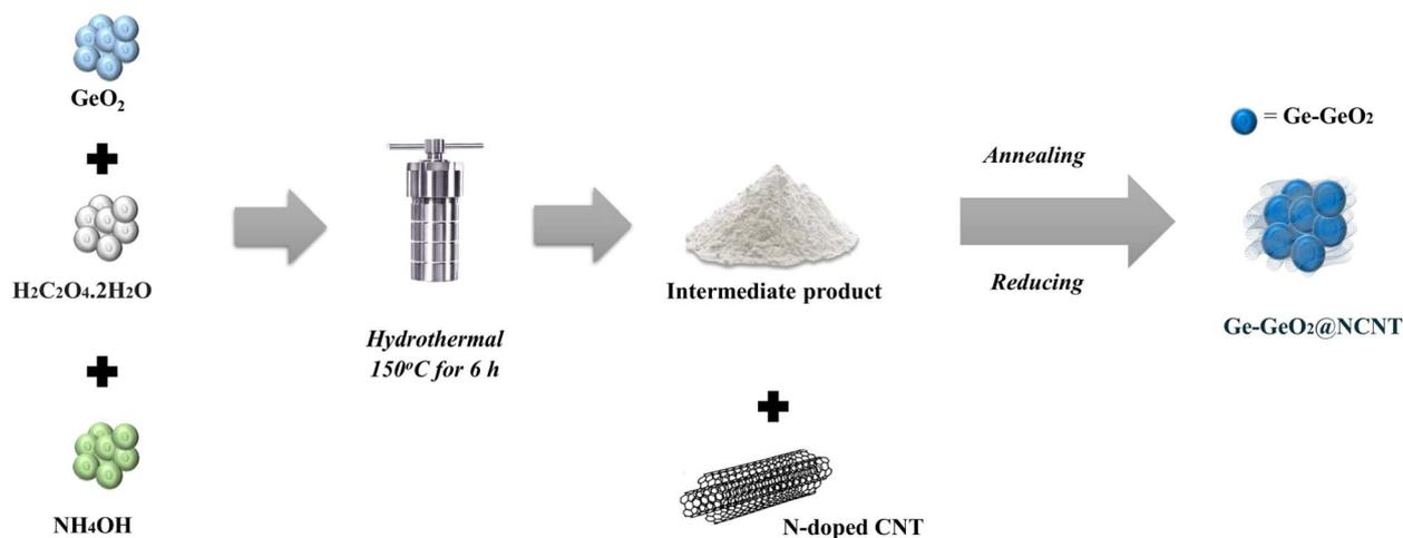
Fig. 1 Schematic of synthesis process of  $\text{GeO}_2\text{-Ge@NCNT}$  composite.
