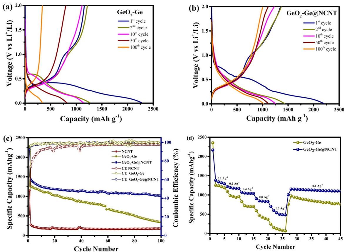
Fig. 7 Charging and discharging profile of (a) GeO<sub>2</sub>-Ge and (b) GeO<sub>2</sub>-Ge@NCNT at 100 mA g<sup>-1</sup>, (c) cycling performance and coulombic efficiency of GeO<sub>2</sub>-Ge and GeO<sub>2</sub>-Ge@NCNT at current density 100 mA g<sup>-1</sup>, and (d) rate performance at different current densities 0.1 A g<sup>-1</sup> to 1.6 A g<sup>-1</sup> for GeO<sub>2</sub>-Ge and GeO<sub>2</sub>-Ge@NCNT.
