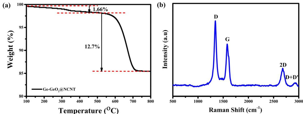
Fig. 3 (a) TGA analysis and (b) Raman spectrum for  $\text{GeO}_2\text{-Ge@NCNT}$ .
