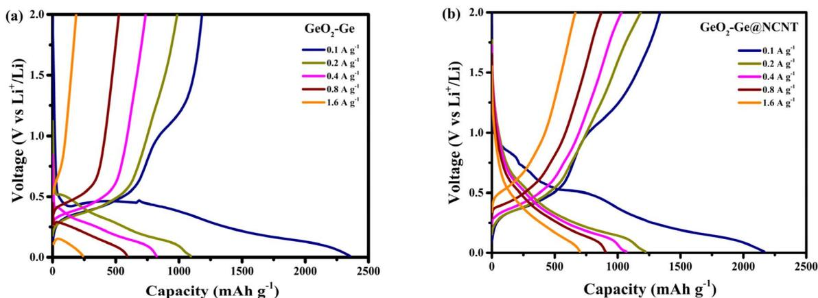
Fig. 8 Charging and discharging profile of (a) GeO<sub>2</sub>-Ge and (b) GeO<sub>2</sub>-Ge@NCNT at different C-rate (0.1–1.6 A g<sup>-1</sup>) in the first cycle.
