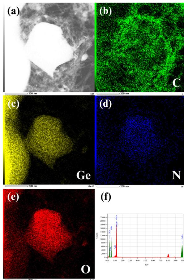
Fig. 6 (a) STEM images and corresponding EDX elemental mapping, indicating (b) C, (c) Ge, (d) N, (e) O signal mapping of  $\text{GeO}_2\text{-Ge@NCNT}$  image, and (f) EDX pattern of  $\text{GeO}_2\text{-Ge@NCNT}$ .
