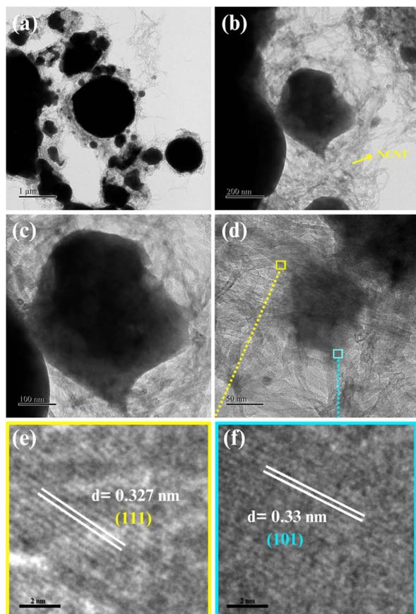
Fig. 5 TEM image of  $\text{GeO}_2\text{-Ge@NCNT}$  in different magnifications: (a) 1  $\mu\text{m}$ , (b) 200 nm, (c) 100 nm, (d) HR-TEM image, and (e and f) lattice fringes of a selected area from image (d).
