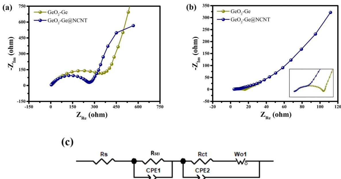
Fig. 11 Nyquist plots of AC impedance for GeO<sub>2</sub>-Ge and GeO<sub>2</sub>-Ge@NCNT (a) before cycling and (b) after 10 cycles, and (c) equivalent circuit model of EIS fitting curve.
