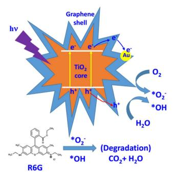
Fig. 10 Illustration of charge transfer in UT@Gr-AuNPs and the proposed photocatalytic degradation mechanism of R6G molecules.
