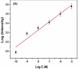
Fig. 7 (a) SERS spectra of R6G molecules with the concentrations of  $10^{-5}$  M to  $10^{-10}$  M adsorbed on UT@Gr-AuNPs samples and (b) the change of peak intensity at 771 cm<sup>-1</sup> as a function of concentration.
