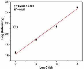
Fig. 12 (a) SERS spectra of different concentrations of malathion and (b) the change of peak intensity at  $724~{\rm cm}^{-1}$  as a function of concentration.
