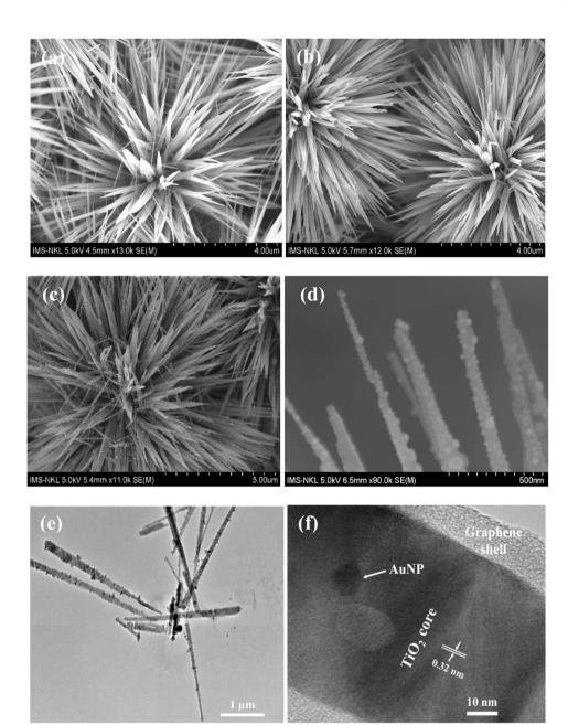
Fig. 1 SEM images of (a) UT, (b) UT@Gr, (c and d) UT@Gr-AuNPs. Typical TEM images (e and f) of UT@Gr-AuNPs.
