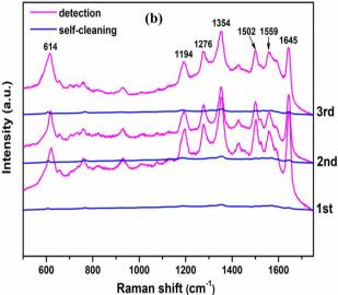
Fig. 11 SERS spectra of: (a) R6G ( $10^{-5}$  M) and (b) RhB ( $10^{-5}$  M) on the UT@Gr-AuNPs before and after self-cleaning for three cycles.
