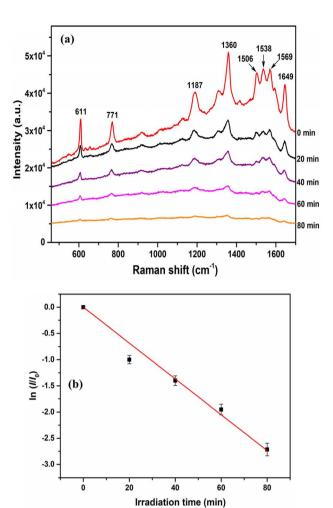
Fig. 9 (a) SERS spectra and (b) linear relationship between the irradiation time and the logarithm of SERS intensities at 771 cm<sup>-1</sup> for the degradation of R6G molecules.
