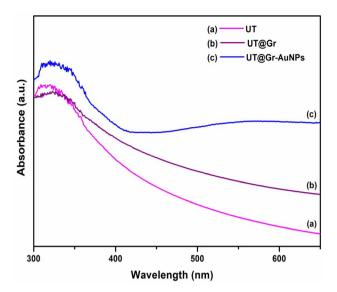
Fig. 5 UV-vis spectra of (a) UT, (b) UT@Gr and (c) UT@Gr-AuNPs samples.
