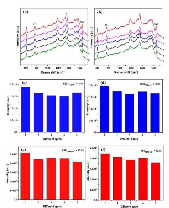
Fig. 8 SERS spectra of  $10^{-5}$  M R6G molecules adsorbed on the surface of UT@Gr-AuNPs for two different batches: (a) batch 1, and (b) batch 2. The RSD values at peaks: 771 cm<sup>-1</sup> for (c) batch 1 and (d) batch 2; 1649 cm<sup>-1</sup> for (e) batch 1 and (f) batch 2.
