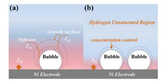
Fig. 6 (a) Growth process of hydrogen bubbles on Ni electrodes. (b) Growth process of multiple bubbles coexisting on Ni electrodes.
