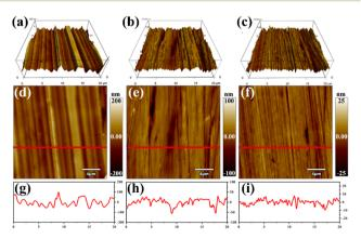
Fig. 4 (a-c) Three-dimensional surface morphology of the Ni electrodes. (d-f) Two-dimensional surface morphology of the three Ni electrodes. (g-i) Height variation distribution of the red lines in (d-f).
