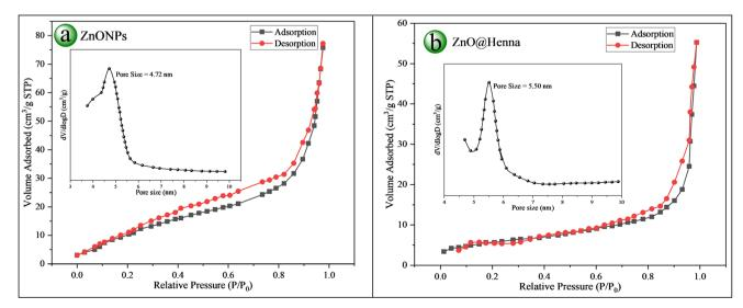
Fig. 10 BET analysis: N<sub>2</sub>-adsorption/desorption isotherms with pore size distribution (inset) of (a) ZnONPs and (b) ZnO@henna nanocomposite.
