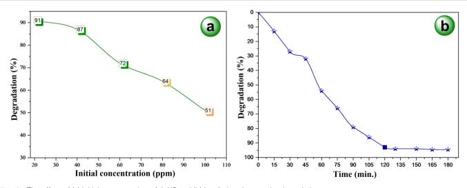
Fig. 12 The effect of (a) initial concentration of 4-NP and (b) irradiation time on the degradation rate.
