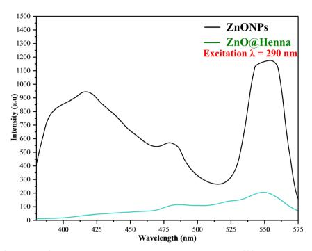
Fig. 9 PL spectra for ZnONPs and ZnO@henna nanocomposite at the excitation wavelength of 290 nm.
