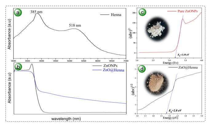
Fig. 7 (a) UV-visible spectra of aqueous henna extract, (b) UV-visible DRS of pure ZnONPs (black line) and ZnO@henna nanocomposite (blue line), (c) band gap energy calculation by DRS analysis for pure ZnONPs, and (d) ZnO@henna nanocomposite.
