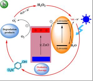
Fig. 15 Illustration of (a) HOMO/LUMO and VB/CB edge potentials of lawsone and ZnONPs, respectively, which shows the favorable electron transfer from the LUMO of lawsone to the CB of ZnONPs. And (b) proposed mechanism for the degradation of 4-NP by ZnO@henna nanocomposite under blue LED illumination.
