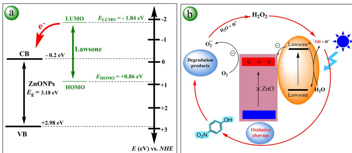
Fig. 15 Illustration of (a) HOMO/LUMO and VB/CB edge potentials of lawsone and ZnONPs, respectively, which shows the favorable electron transfer from the LUMO of lawsone to the CB of ZnONPs. And (b) proposed mechanism for the degradation of 4-NP by ZnO@henna nanocomposite under blue LED illumination.
