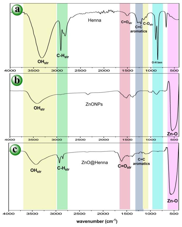
Fig. 4 The functional group analysis for (a) henna aqueous extract, (b) ZnONPs, and (c) ZnO@henna nanocomposite.
