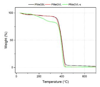
Fig. 3 Thermogravimetric analysis results of polymer samples.
