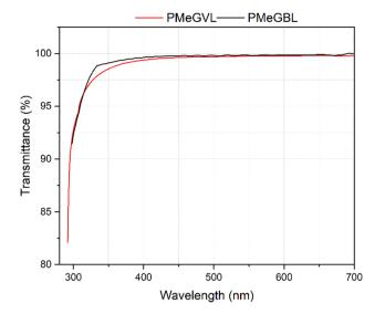
Fig. 5 Transmittance measurement of casted polymer films within 300–700 nm range.
