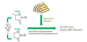
**Scheme 1** Depiction of synthetic methodology to manufacture acrylic-type renewable polymers *via* radical polymerization in renewable solvents.
